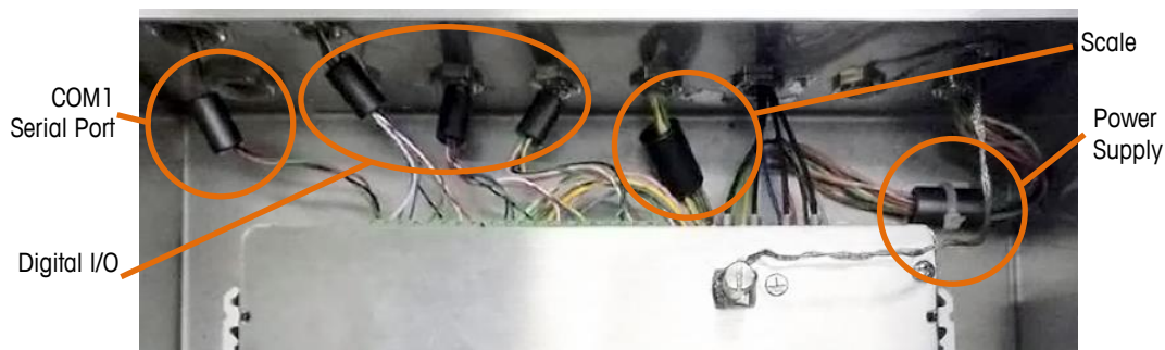
Figure A-15: Ferrites Required for SICSpro Panel Installation
