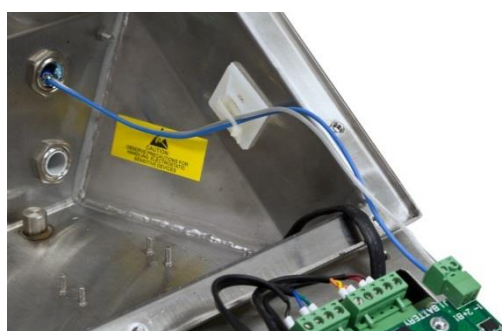
Figure A-32: PAB Battery Pack Connector (left) and Battery Cable Installation
