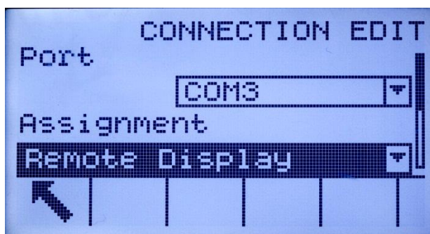
Figure 3-13: COM2/COM3 Connection Configured for Remote Operation
