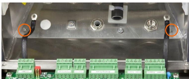
Figure A-12: Additional Studs for Alternative Attachment of Cover
