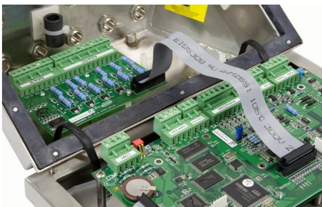
Figure A-34: Harsh Enclosure Discrete I/O Installation
