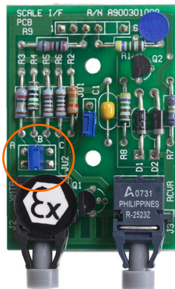
Figure A-43: J2 Pin Location on Puma/ID3sTx FO Option PCB
