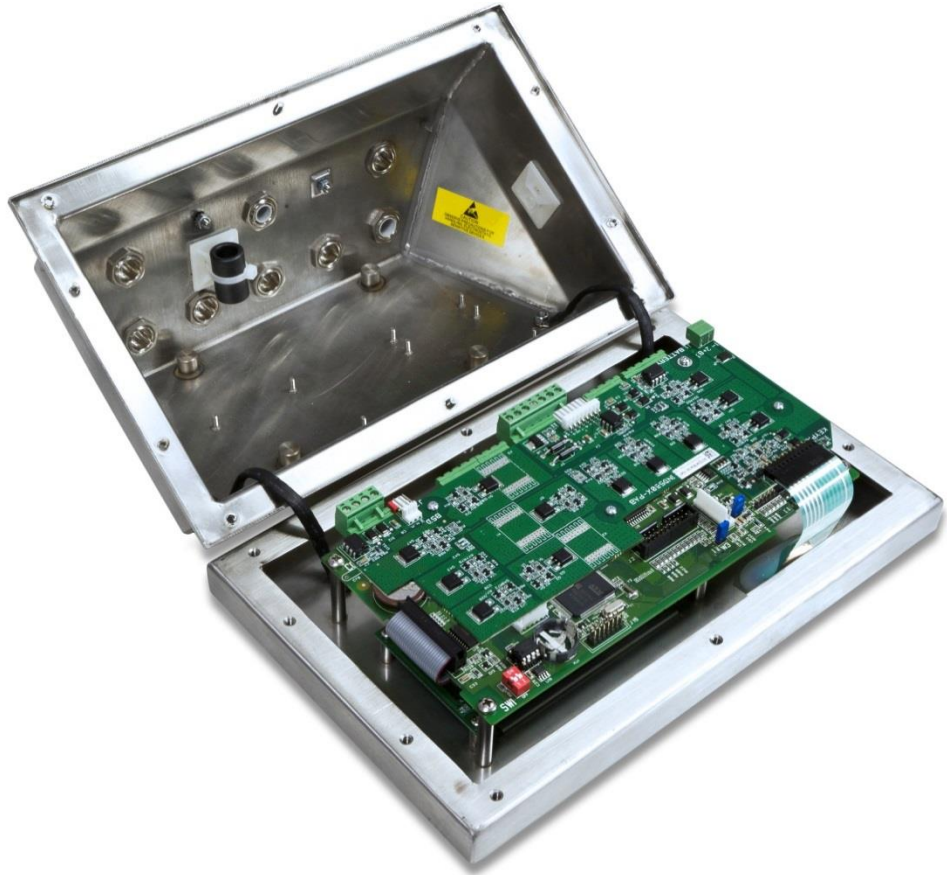
Figure A-28: PAB Installed on IND560x Main Board
