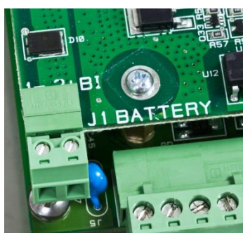
Figure A-32: PAB Battery Pack Connector (left) and Battery Cable Installation
