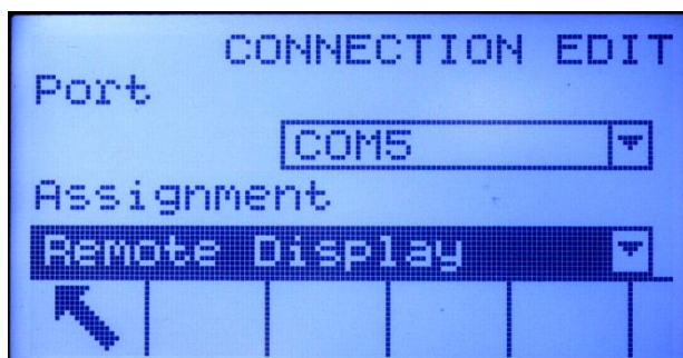
Figure 3-15: COM4 or COM5 Connection Configured for Remote Operation
