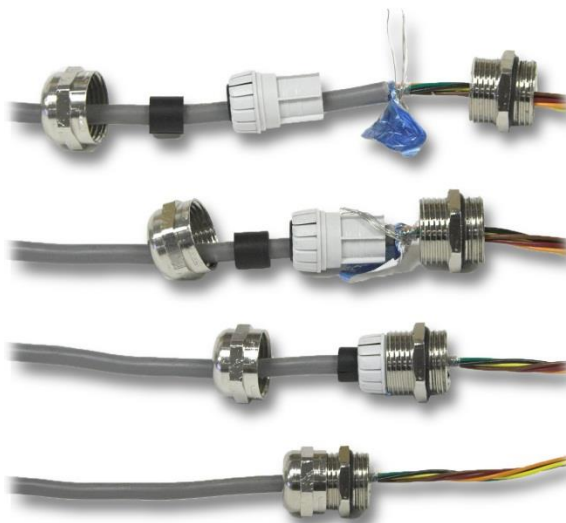
Figure A-17: Shield Termination at Gland
