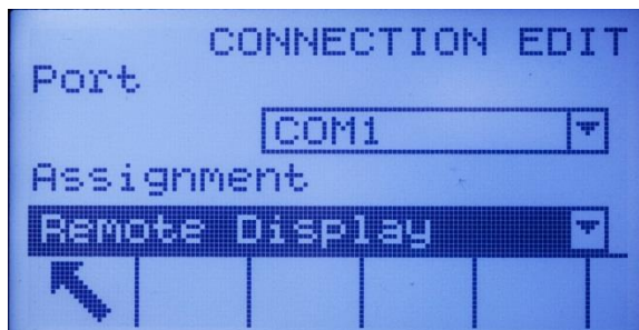
Figure 3-11: COM1 Connection Configured for Remote Operation
