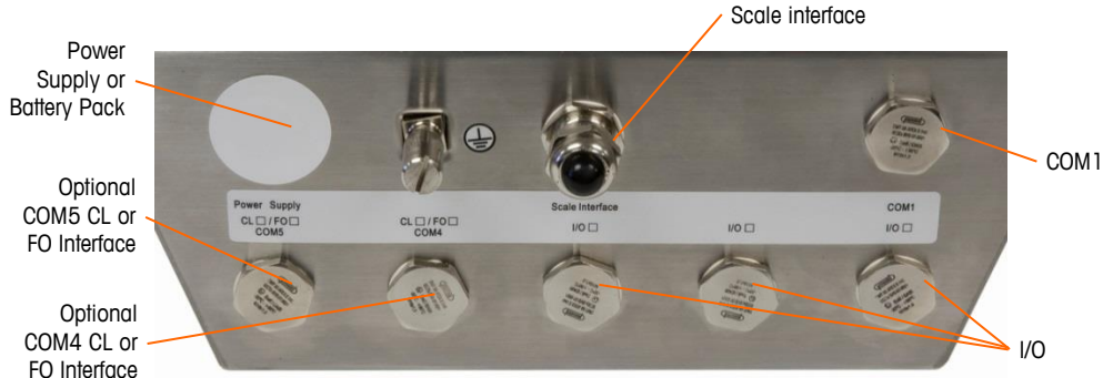
Figure A-16: Cable Gland and Plug Assignments
