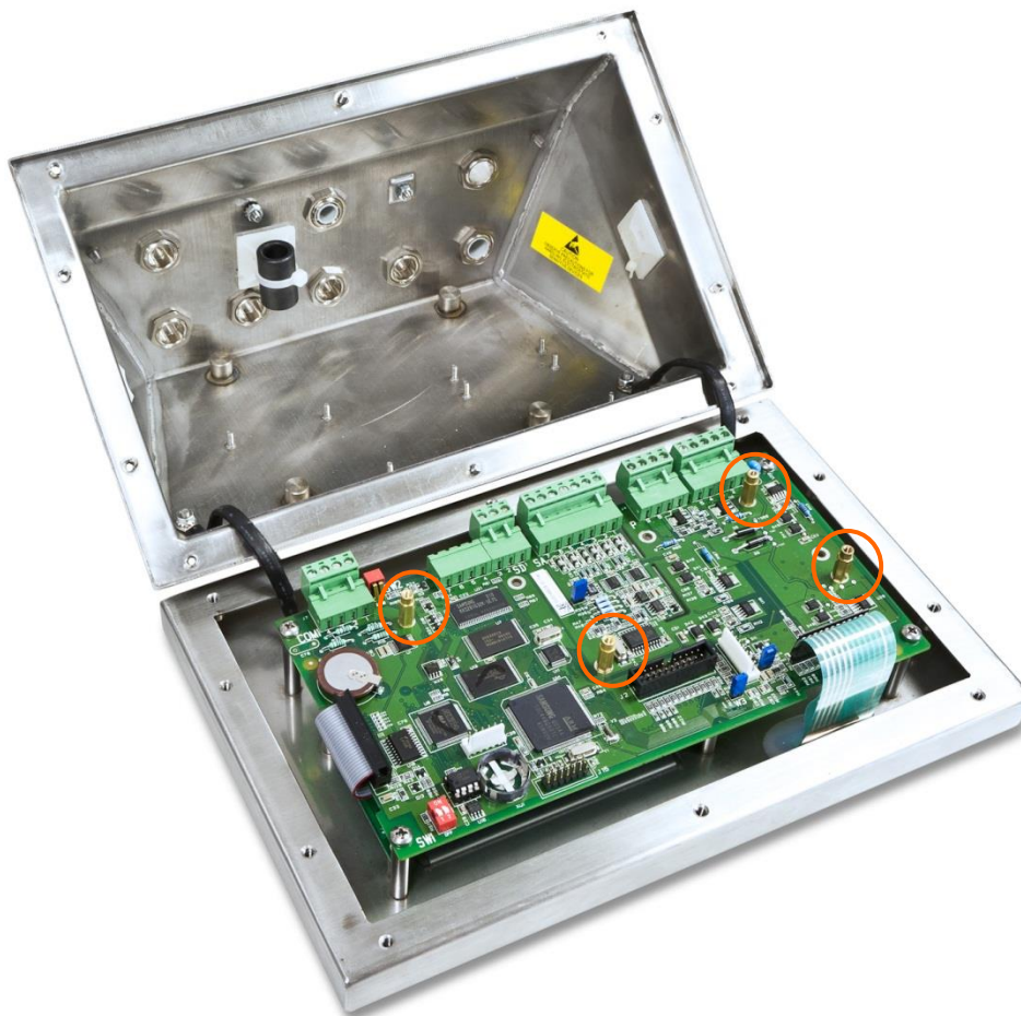
Figure A-27: Location of IND560x-PAB Brass Standoffs
