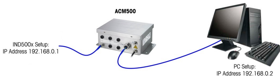
Figure 177: Example: IP Address Configuration (Crossover or Hub Configuration)
