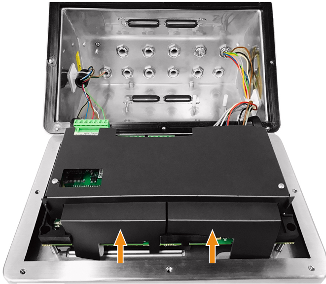
Figure 51: Reinstall the Plastic Protective Cover
