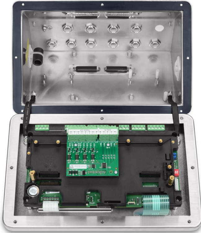
Figure 32: Discrete IO Interface, installed
