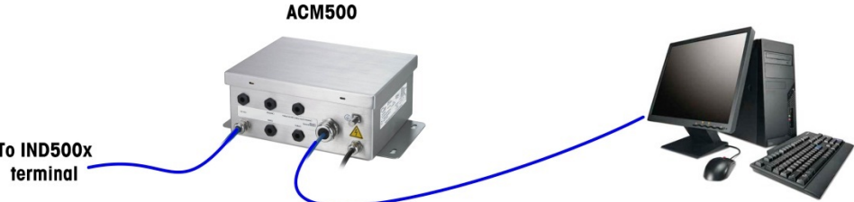
Figure 123: Connection with Crossover Cable
