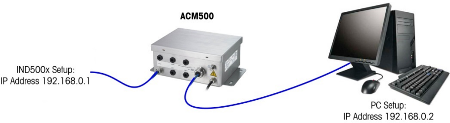
Figure 125: Example: IP Address Configuration (Crossover or Hub Configuration)
