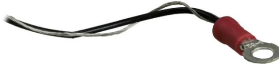
Figure A-63: Ring Terminal Crimped to Black and Drain Wires
