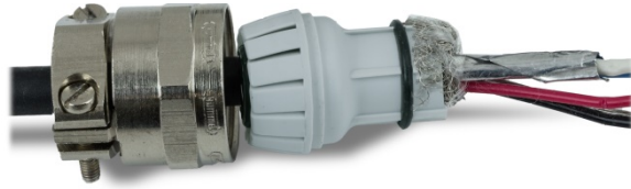
Figure A-62: Inner Shield Unbraided and Folded Back over Grommet
