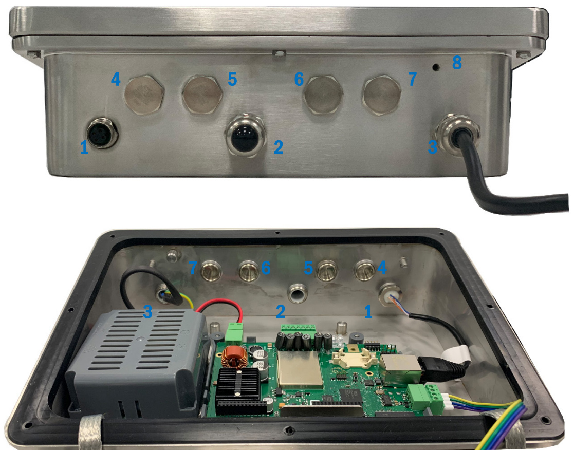
Figure A-25: Harsh Enclosure Cable Opening Assignments (External and Internal Views)
