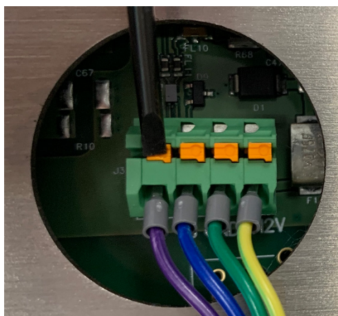
Figure A-17: Orange levers on display board connector
