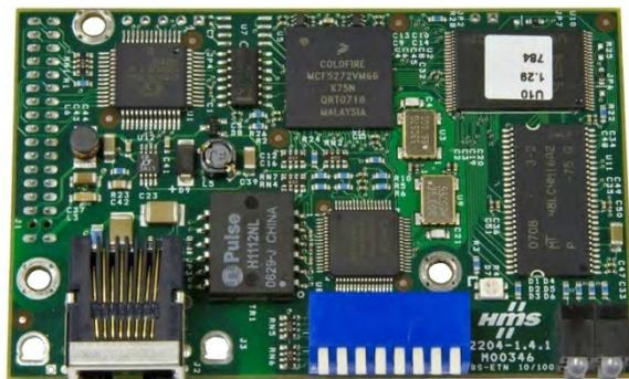
Figure A-59: Ethernet / IP Option Board
