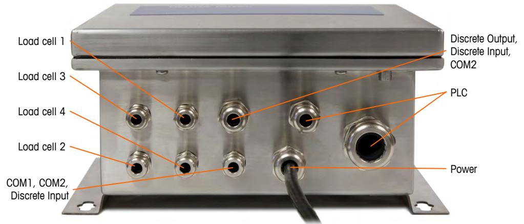
Figure A-25: J-Box Enclosure Gland Assignments
