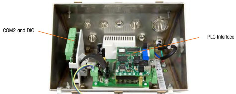
**Figure A-39: Option Locations in the Harsh Enclosure**
