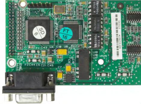
**Figure A-55: PROFIBUS Option Board, Panel Mount Enclosure**
