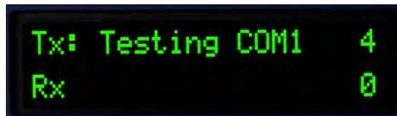
Figure 4-3: Serial Test Display
