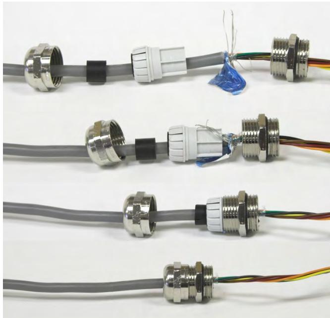
Figure A-26: Cable Shield Grounding
