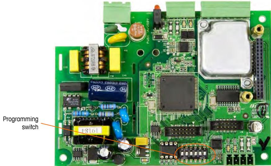
Figure A-61: Main PCB DIP Switch Array
