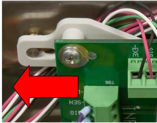
**Figure A-32: Removing the Summing Board**
