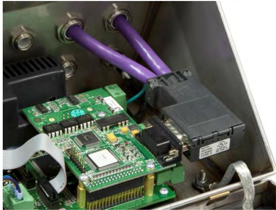
Figure A-57: Harsh Enclosure PROFIBUS Cable Routing
