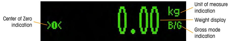
Figure 2-1: Display in Weighing Mode
