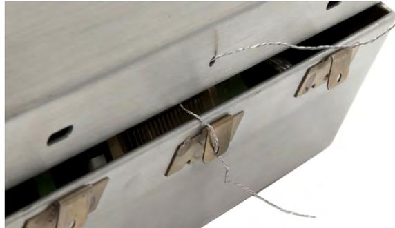
**Figure A-67: Harsh Enclosure Sealing, Wire Routing**
