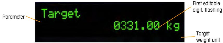
Figure 2-7: Target Entry Screen, Value in Focus
