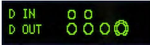
Figure 3-17: Discrete I/O Test Display, Output Active (bottom)
