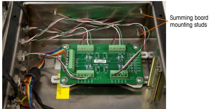
**Figure A-33: IND131 Terminal Removed, Summing Board in Position for Wiring**
