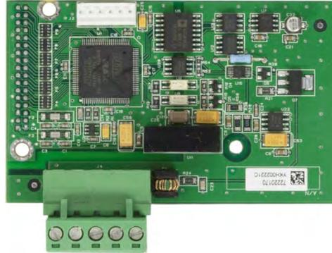
Figure A-49: Analog Output Option Board
