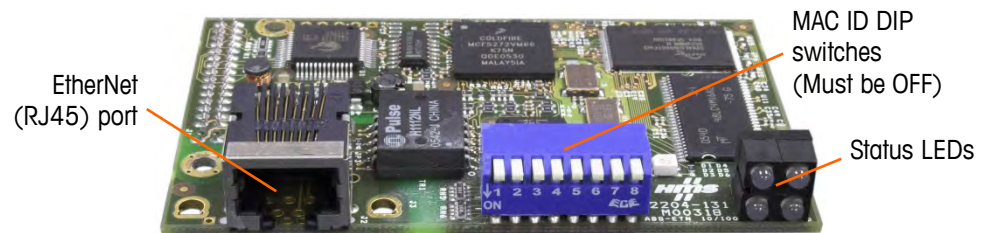
Figure 6-2: EtherNet / IP Module Components
