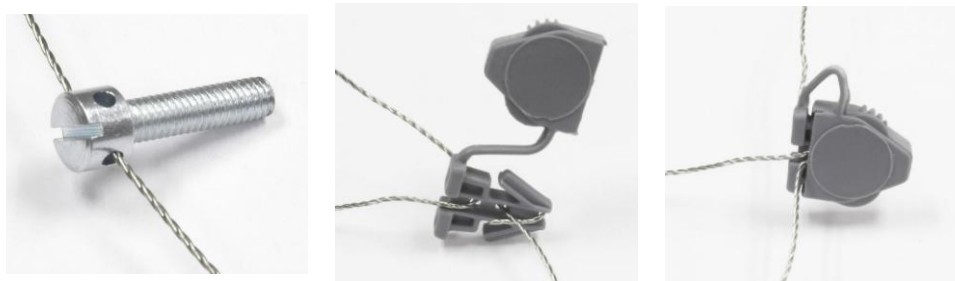
Figure A-72: Use of the Sealing Kit: Wire Through Screw (left), Wire Through Seal (center), Seal Closed (right)
