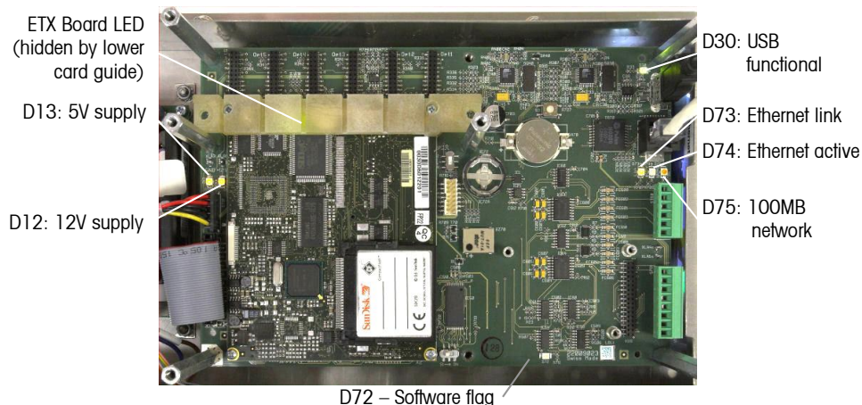
Figure 4-8: Main PCB LEDs
