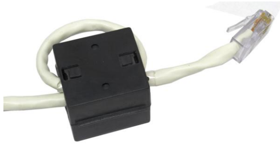
Figure A-16: Installing Clamp Ferrite
