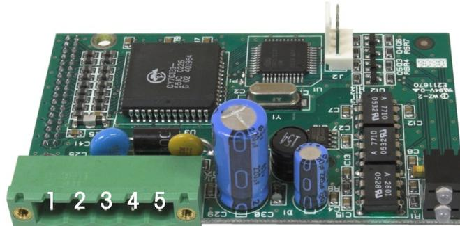
**Figure 5-4: DeviceNet Connector Pin Numbering**
