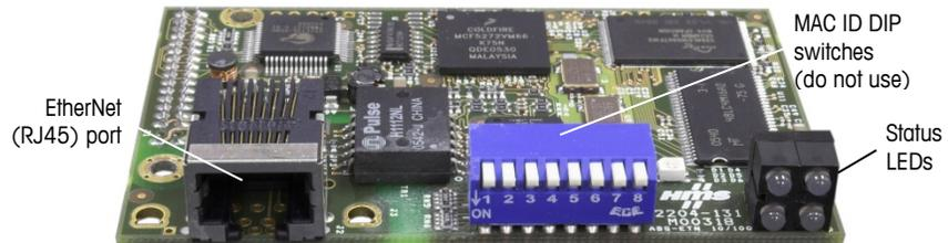
Figure 6-2: Ethernet / IP - Modbus TCP Option Board Components
