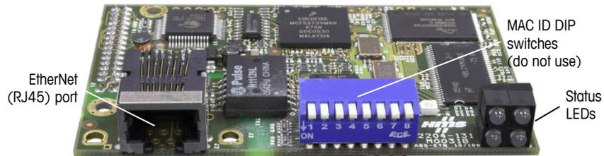
Figure 4-2: EtherNet / IP Module Components
