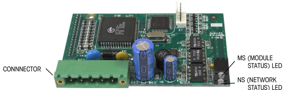
**Figure 5-2: DeviceNet Option Board Components**
