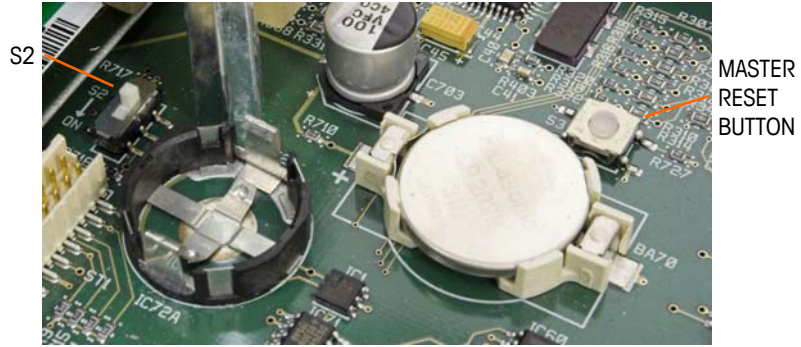
Figure 3-51: Main PCB, Master Reset Button and S2 Locations Indicated
