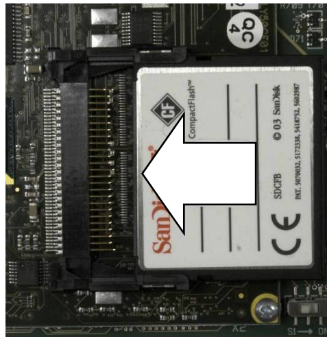
Figure 3-62: CF Card Installation
