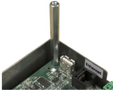
Figure 3-54: Stand-Off on Main PCB
