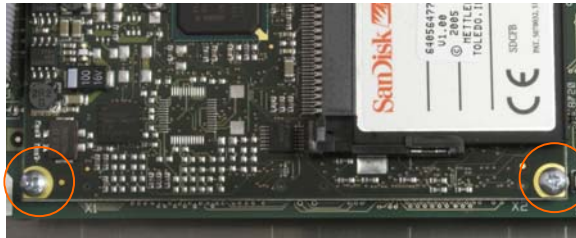
Figure 3-56: ETX Board Mounting Screws
