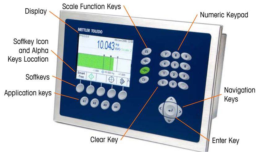
Figure 2-2: Front Panel Components and Key Locations
