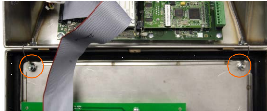
Figure A-7: Ground Strap Attachment Locations
