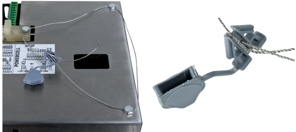
Figure A-111: Sealing Wire Installed, Wire Threaded Through Seal
