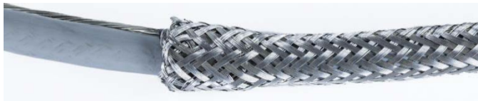
Figure A-53: Outer Sheath Pushed Up Over Taped End
