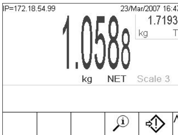
Figure 2-17: Class II-Approved IDNet Base Weight Display
