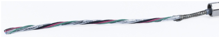
Figure A-56: Inner Sheath Trimmed Back
