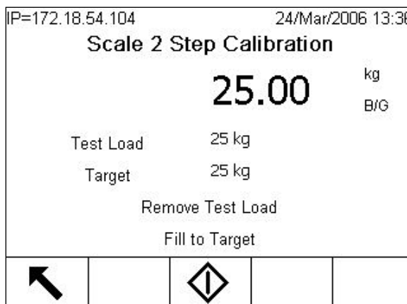
Figure 3-32: Step Calibration, First Step Complete
