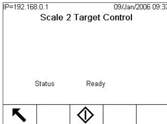
Figure 2-18: Example of Ready State in Target Control
