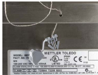
Figure A-115: Sealing Wire Threaded Through Cover and Clip
