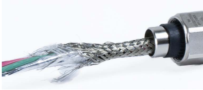
Figure A-57: Inner Sheath Frayed
