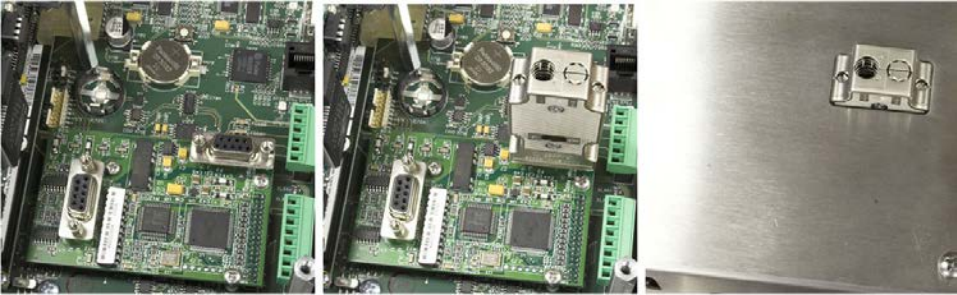
Figure A-104: Profibus PLC Module Connector for Panel Mount Enclosure
