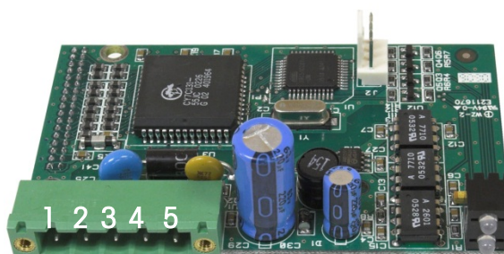
Figure A-97: DeviceNet Option Board Connector Pin Numbering
