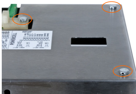
Figure A-110: Panel Enclosure Rear Cover with Sealing Screws Installed
