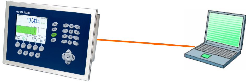
Figure D-1: Connecting the IND780 to a PC with a Crossover Cable
