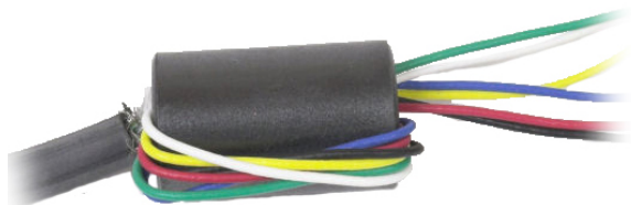
Figure A-16: Ferrite Core on Analog Load Cell Cable
