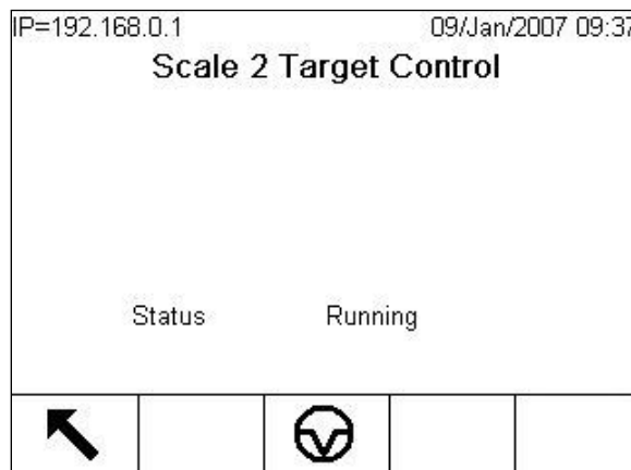
Figure 2-19: Example of Running State in Target Control
