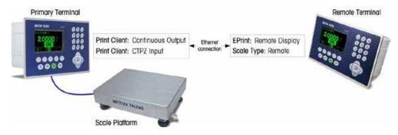
Figure 4-9: Example of Terminal Configuration for Remote Display Function via Ethernet
