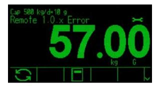
Figure 2-34: Asynchronous Error System Line Message
