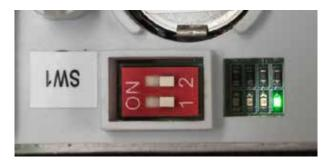
Figure 5-11: Position of LED 4 on Main Board PCB
