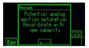
Figure 3-6: Analog Saturation Warning
