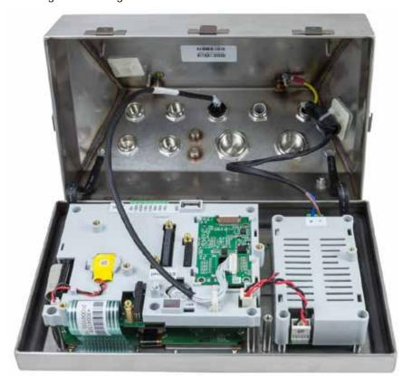
Figure A-13: Front Panel and Load Cell Connection Reversed
