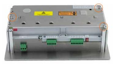
Figure A-1: Opening the Panel-Mount Enclosure
