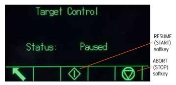
Figure 2-19: Example of Paused State in Target Control
