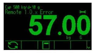
Figure 5-5: Asynchronous Error System Line Message
