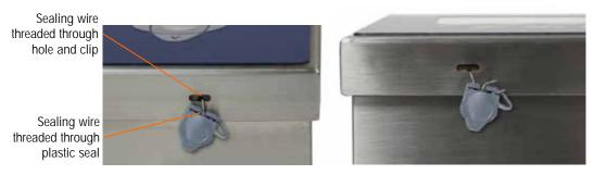
Figure A-61: Harsh Enclosure Seal Threaded and Ready to be Closed – Standard Orientation (left) and with Panel Reversed (right)
