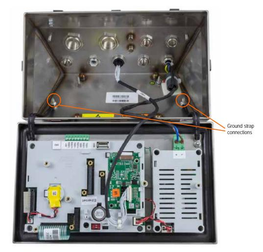
Figure A-11: Loosening the Ground Straps
