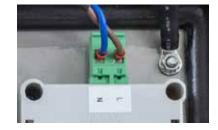
Figure 5-13: AC Power Test Point - Panel (left) and Harsh (right)
