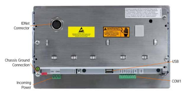
Figure A-21: Panel Mount Enclosure Connections, including IDNet Scale Interface
