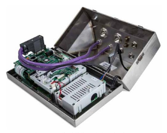
Figure A-48: Profibus Cable Connection in Harsh Enclosure
