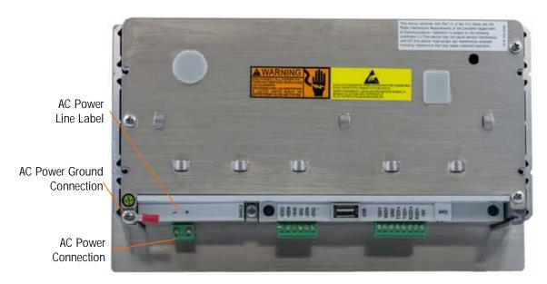
Figure A-23: AC Power Connection on Panel Mount
