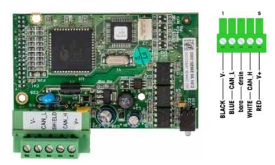
Figure A-44: DeviceNet PLC Option Board and Wiring
