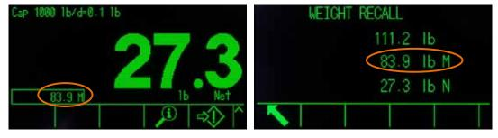
Figure 2-15: Tare Displays with Net Sign Correction Enabled
