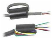
Figure A-15: Installing the Ferrite Cores
