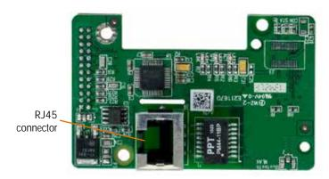
Figure A-31: Ethernet Connection Option Board
