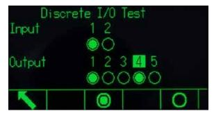
Figure 5-16: Discrete I/O Test Screen
