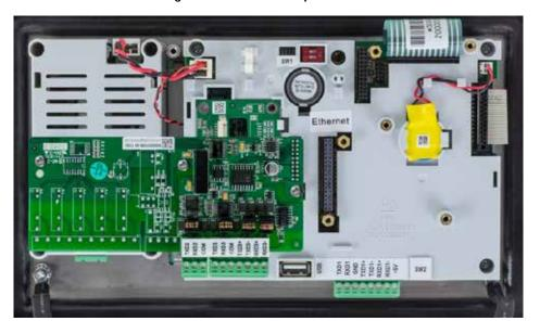
Figure A-35: COM2/3 Option Board, Installed
