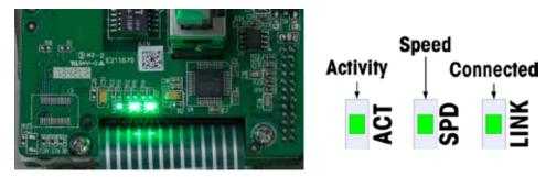
Figure 5-12: Ethernet TCP/IP LEDs
