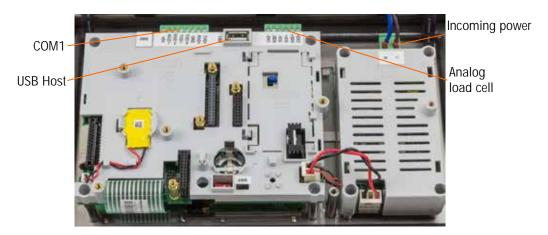
Figure A-20: Analog Main Board in Harsh Enclosure
