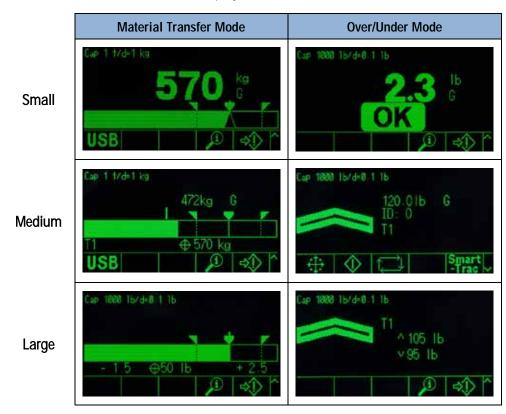
Figure 3-7: SmartTrac Display Sizes, Material Transfer and Over/Under Modes
