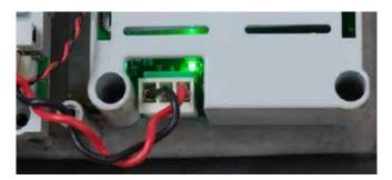
Figure 5-10: 12-VDC LED on Power Supply
