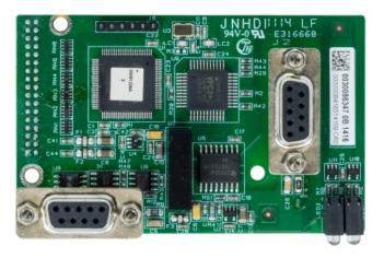
Figure A-47: Profibus Option Board for Harsh Enclosure
