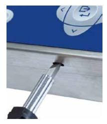
Figure A-2: Opening the Harsh Enclosure
