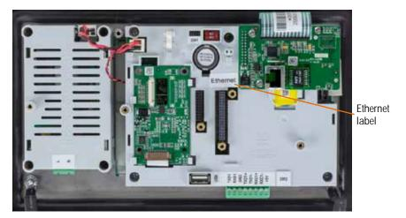
Figure A-32: Ethernet Option Installed on Main Board
