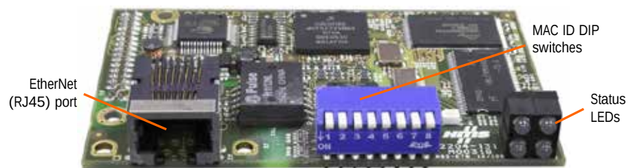
Figure 5-1: EtherNet/IP - Modbus TCP Option Board Components
