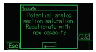
Figure 3-6: Analog Saturation Warning
