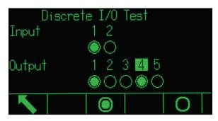
Figure 5-8: Discrete I/O Test Screen
