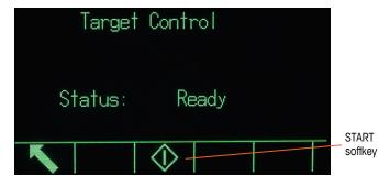
Figure 2-17: Example of Ready State in Target Control
