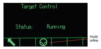
Figure 2-18: Example of Running State in Target Control
