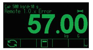
Figure 2-34: Asynchronous Error System Line Message
