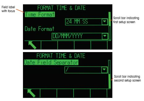
Figure 3-3: Examples of Setup Screens (Format Time & Date)
