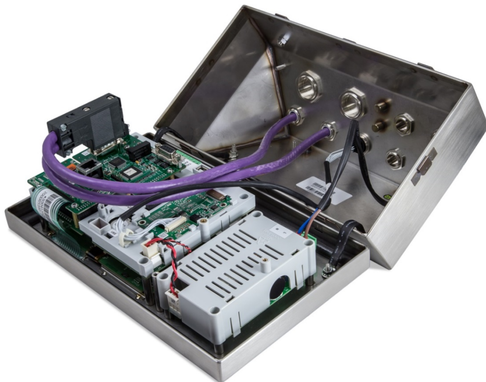
Figure A-110: PROFIBUS Cable Connection in Harsh Enclosure
