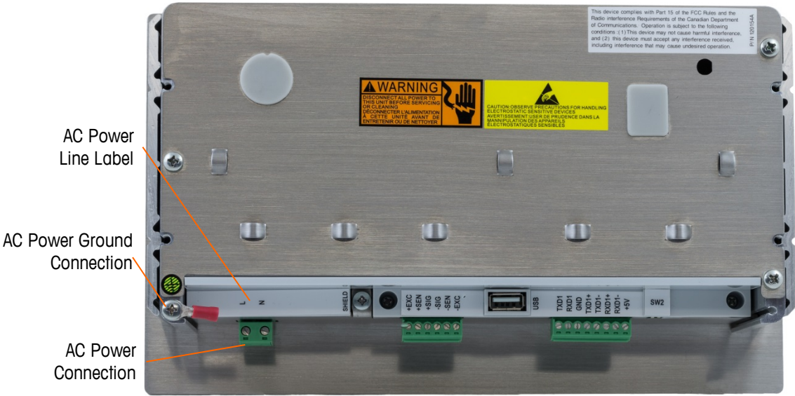
Figure A-27: AC Power Connection on Panel Mount
