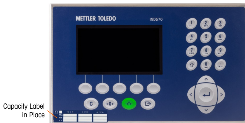
Figure A-119: Capacity Label Installed
