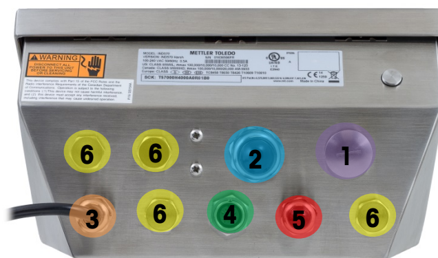
Figure A-19: Harsh Enclosure Cable Opening Assignments
