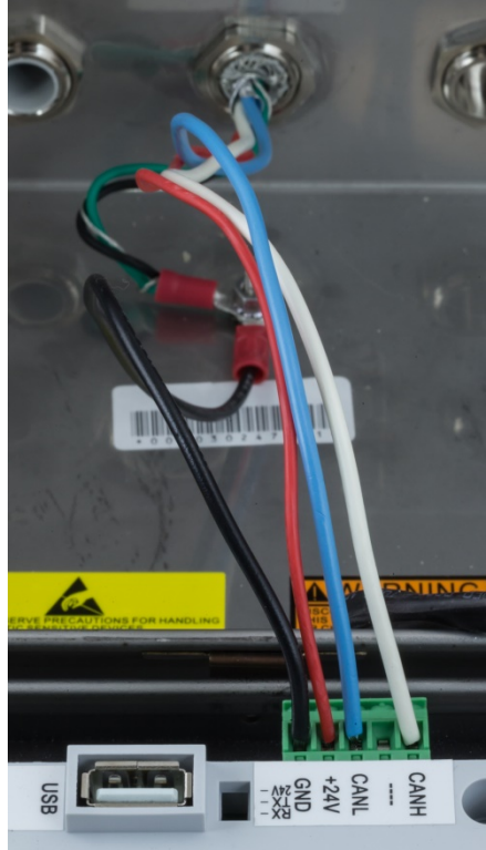
Figure A-55: POWERCELL Wires Connected in Terminal
