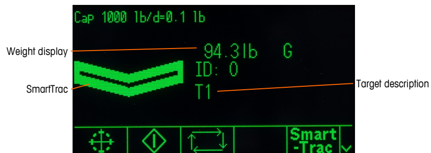
Figure 2-27: Over/Under Display, Medium
