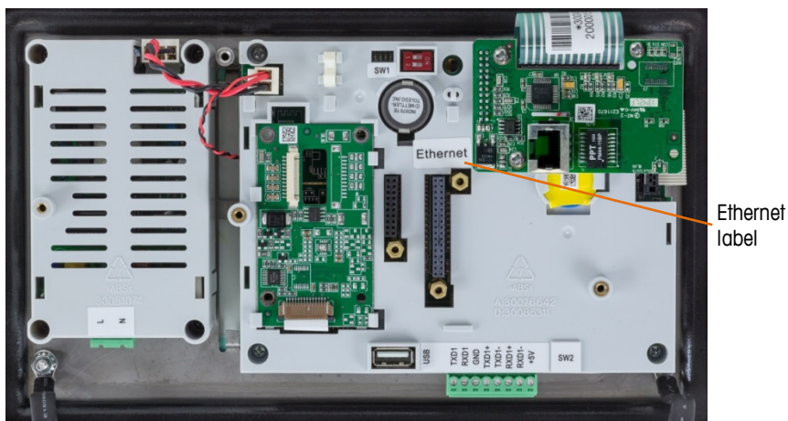
Figure A-90: Ethernet Option Installed on Main Board
