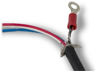
Figure A-76: Ring Terminal Crimped onto Black and Drain Wires
