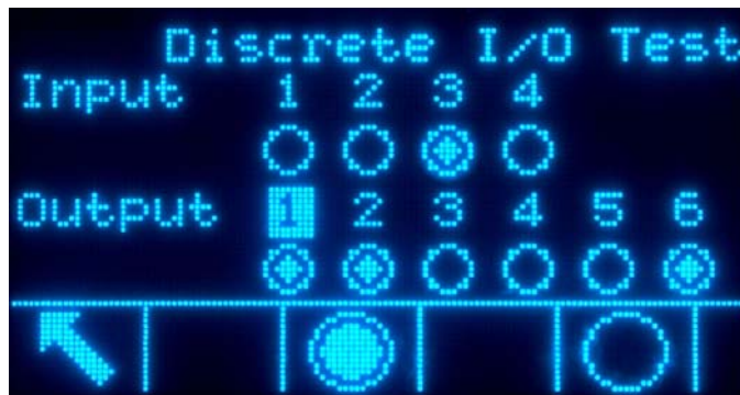
Figure 4-5: Discrete I/O Test Screen
