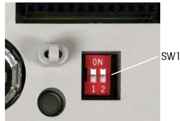
Figure 4-6: Switches SW1-1 and SW1-2
