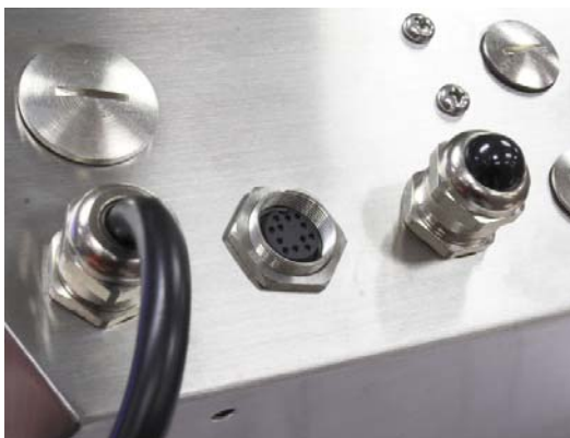
Figure A-18: IDNet Connector Location on the Harsh Enclosure
