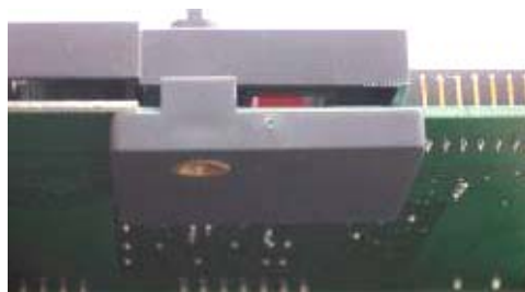
Figure A-54: Attaching the Plastic Bottom Sealing Plate
