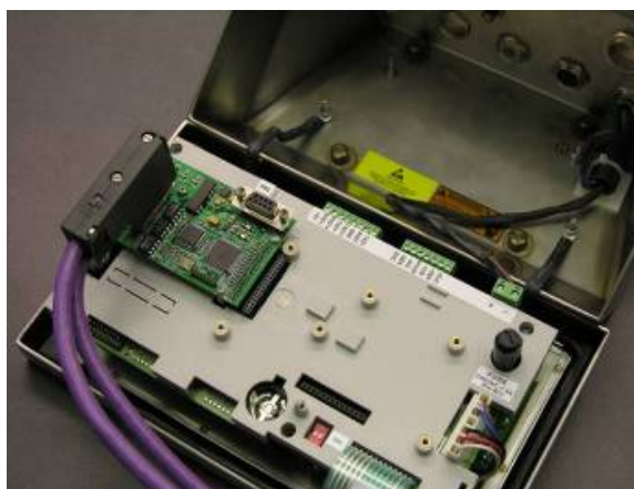
Figure A-40: PROFIBUS Cable Connection in Harsh Enclosure
