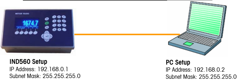
Figure D-3: IP Address Configuration Example (for Crossover or Hub Configuration)
