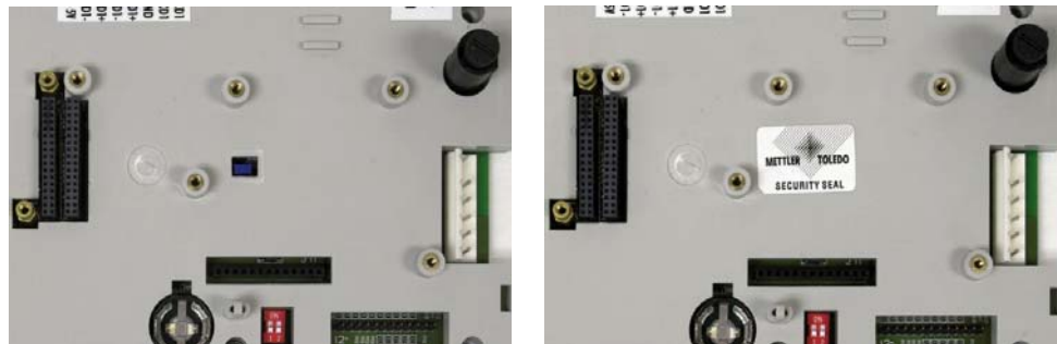
Figure A-57: W1 Millivolt Jumper – Unsealed (left) and Sealed (right)
