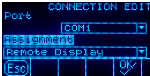
Figure 3-8: Connection Configured for Remote Operation
