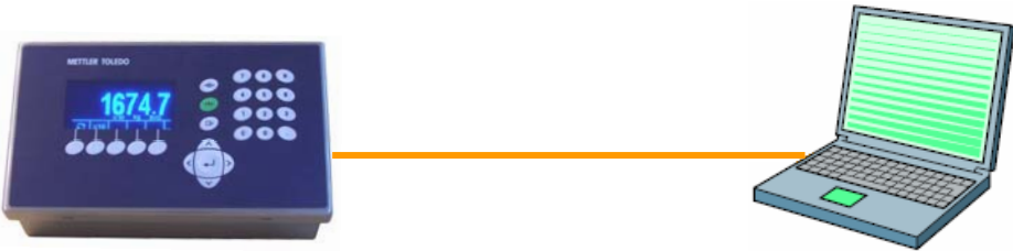
Figure B-1: Connecting the IND560 to a PC with a Crossover Cable
