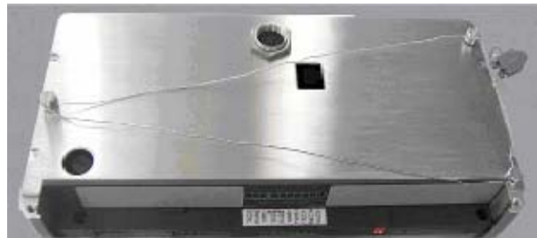
Figure 2-37: External Sealing for Canada
