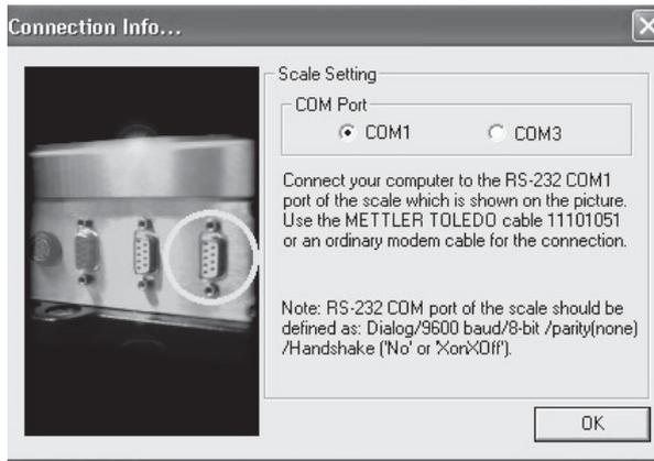
You will then be prompted to connect the interface cable to the first serial interface of the scale (COM1).
