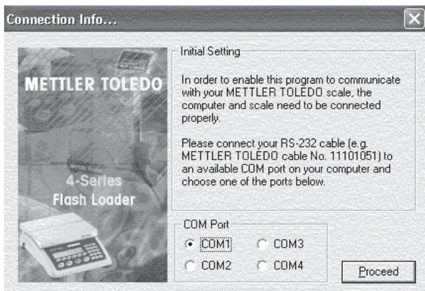
Start the FlashLoader. **The first time it is started** it prompts you to select the interface of the PC to which the scale is connected.
