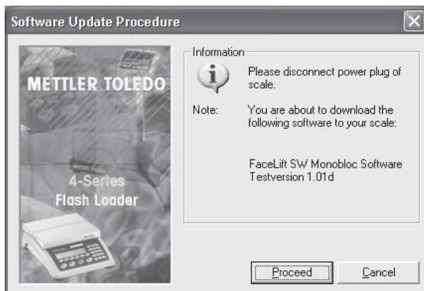
De-energize scale or terminal (disconnect power plug) and confirm with "Proceed".
