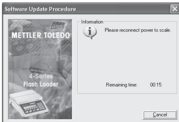
After loading, reconnect the scale or terminal to the power supply.
