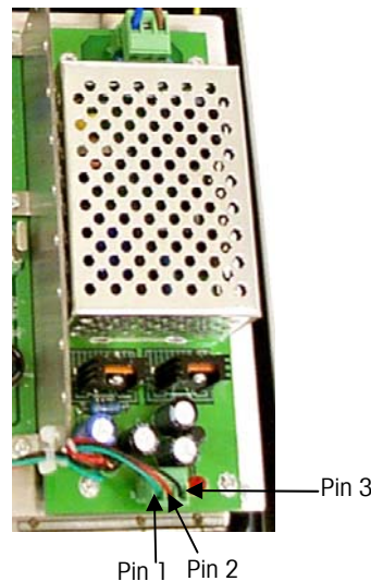
Figure 4-1: Pins 1, 2, and 3 on the Power Supply Board
