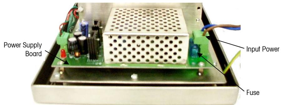
**Figure A-5:** Power Supply Board
