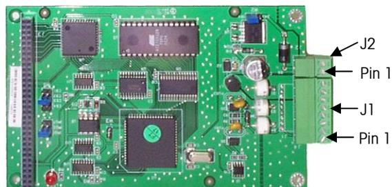
**Figure A-9:** POWERCELL Board Connector Locations
