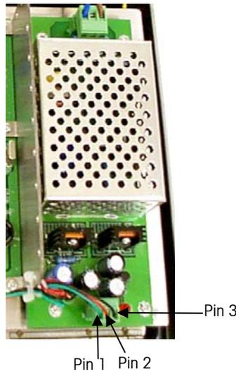
**Figure 4-1:** Pins 1, 2, and 3 on the Power Supply Board
