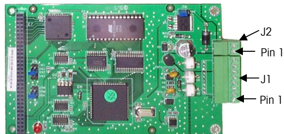
Figure 2-8: POWERCELL Board Connector Locations
