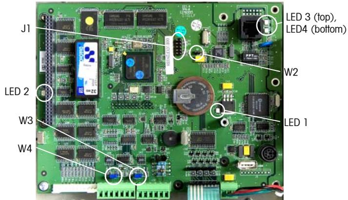
**Figure A-13: Jumper and LED Locations, Original Main PCB**
