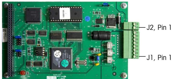
**Figure A-9: POWERCELL Board Connector Locations**
