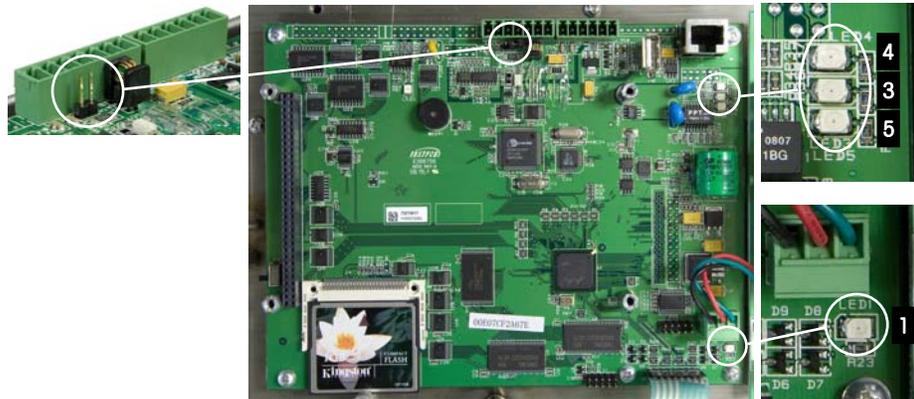
**Figure A-14: Revised Main PCB – Locations of Jumper W1 (left) and LEDs (right)**
