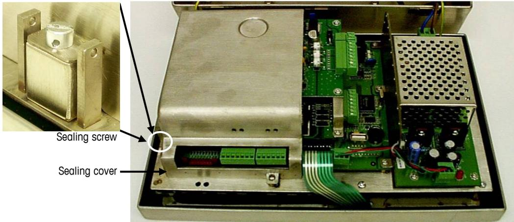
**Figure A-17: Internal Sealing, Original PCB**
