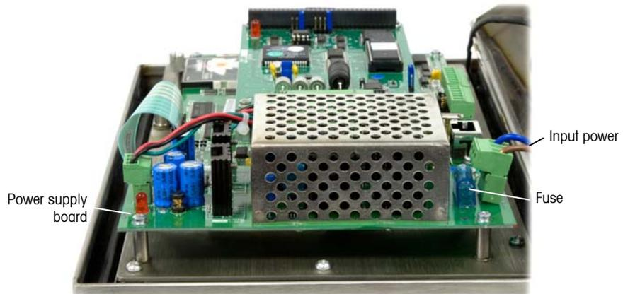
**Figure A-5: Power Supply Board**
