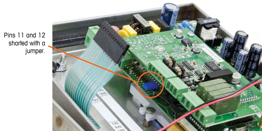
Figure 5-4: Jumper Test for On/Off Key
