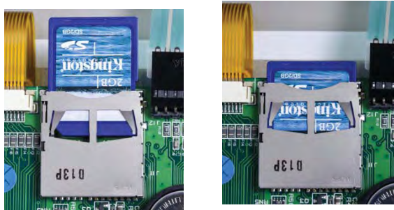
Figure A-33: Sliding an SD Card into the SD Socket (left); SD Card Installed (right)
