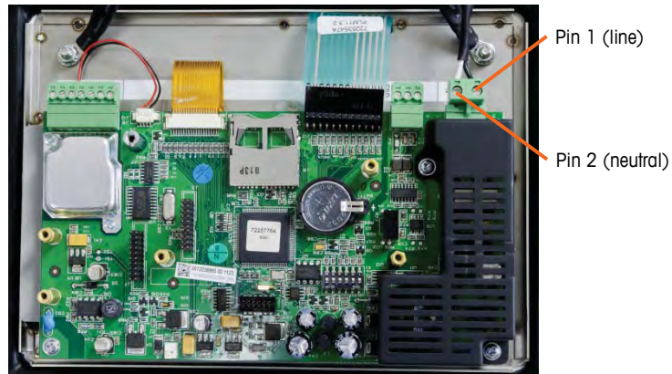
Figure 5-5: Pin Locations for AC Power Test
