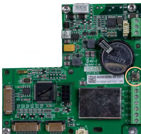
Figure 3-2: Setup Switch Location on Terminal Main Board
