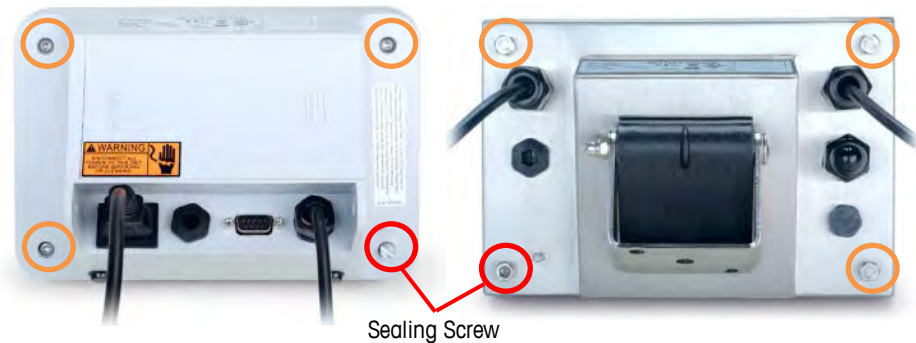
Figure A-2: Opening the Enclosures – IND231 (left) and IND236 (right)
