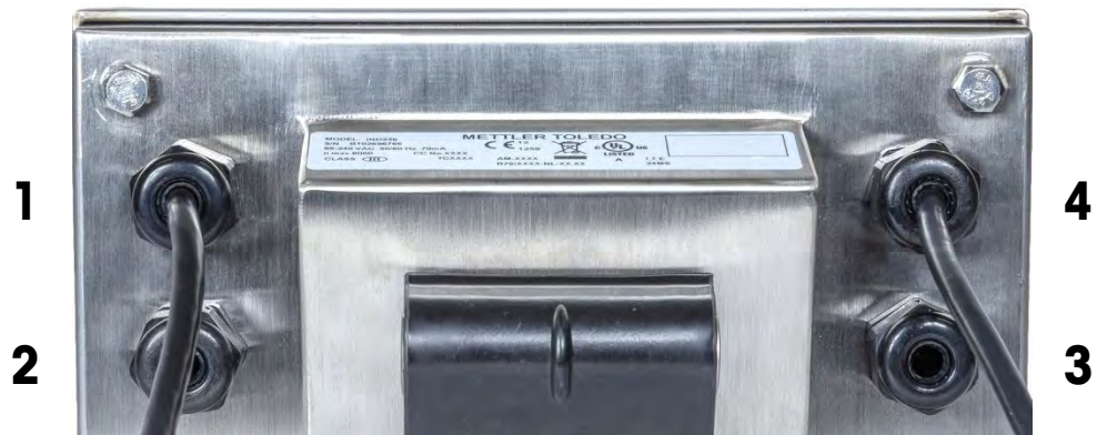
Figure A-14: IND236 Enclosure Openings
