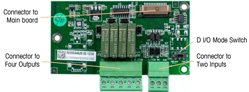
Figure A-36: Discrete I/O Option Board
