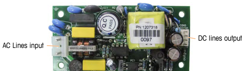
Figure A-17: Power Board
