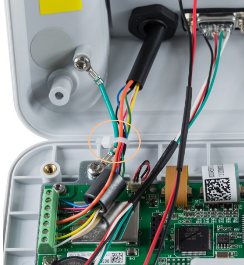
Figure A-20: Analog Load Cell Pin Grounding and Ferrite Installation, IND231
