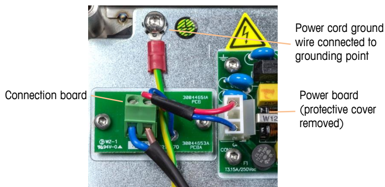
Figure A-18: IND236 AC Power Connection Board and Grounding
