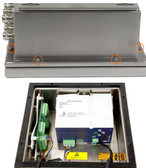
Figure 2-2: J-Box Enclosure, Original
