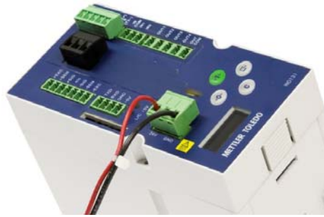
Figure 2-32: DC Power Connection
