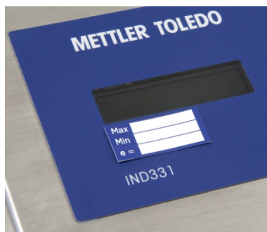
Figure 2-74: Capacity Label Location, Harsh Unit
