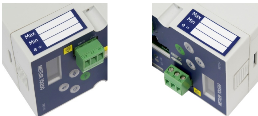
Figure 2-73: Capacity Label Locations, DIN Unit
