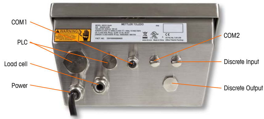
Figure 2-25: Harsh Enclosure Gland Assignments
