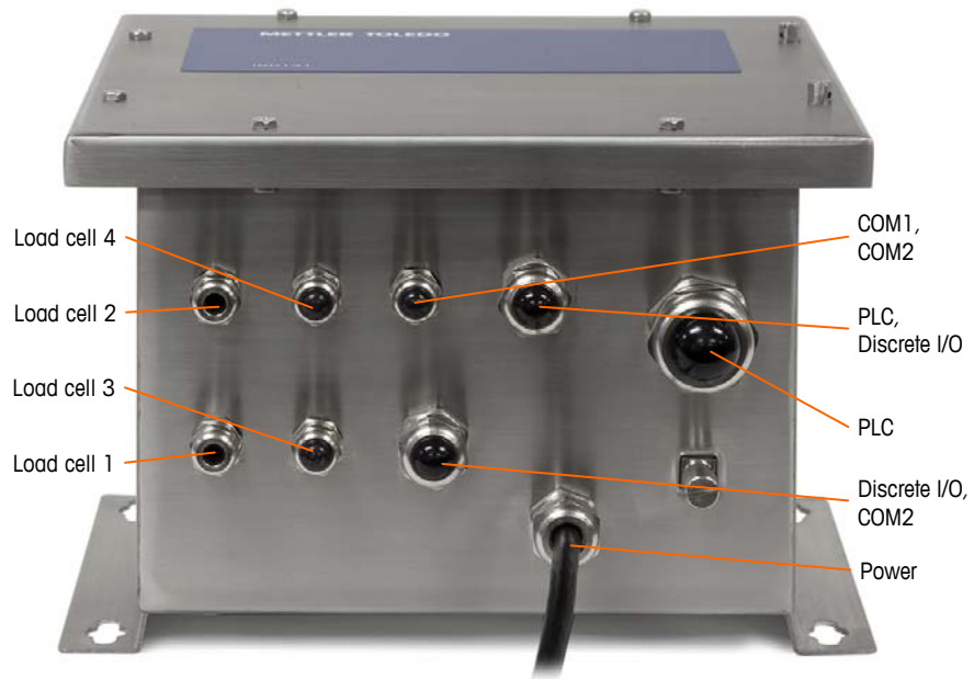
Figure 2-27: Updated J-Box Enclosure Gland Assignments
