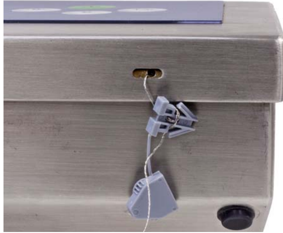
Figure 2-77: Harsh Enclosure Sealing, Wire Routing
