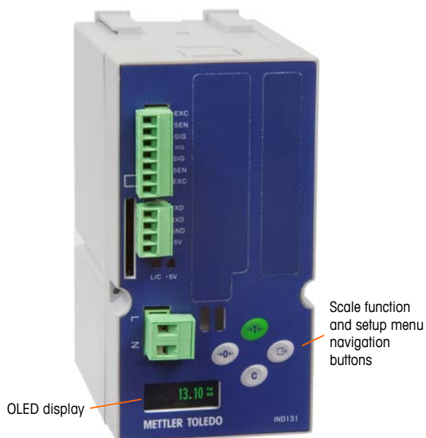
Figure 1-8: IND131 Front Panel Layout
