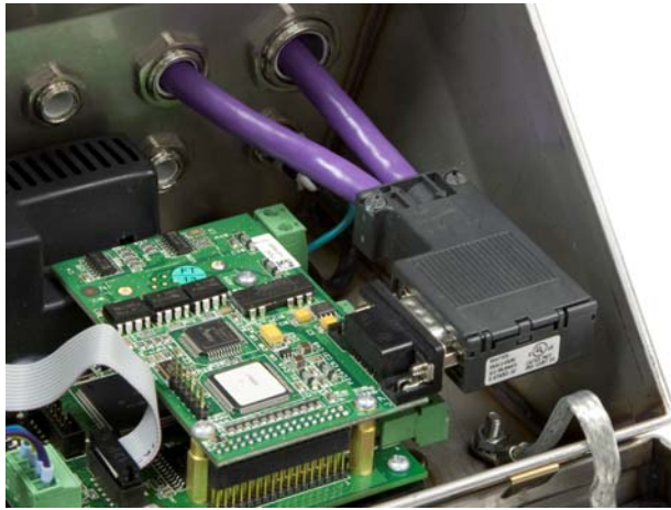
Figure 2-61: Harsh Enclosure PROFIBUS Cable Routing
