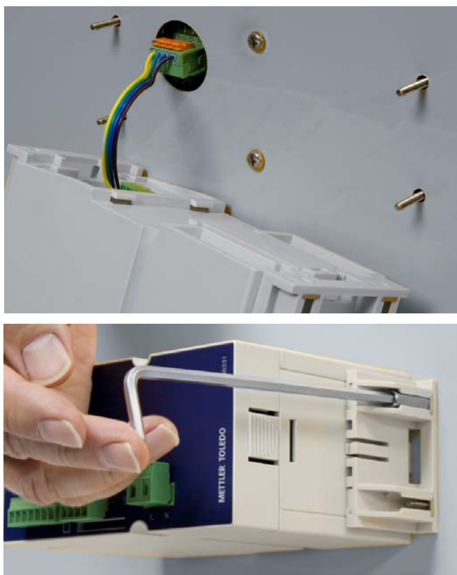
Figure 2-14: Installation du module DIN
