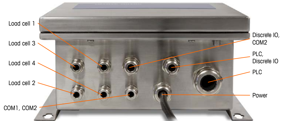
Figure 2-26: Original J-Box Enclosure Gland Assignments
