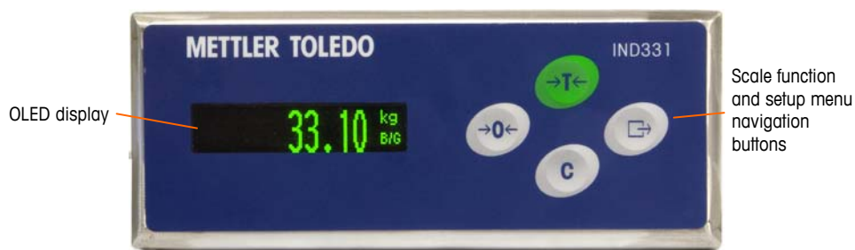
Figure 1-9: IND331 Front Panel Layout
