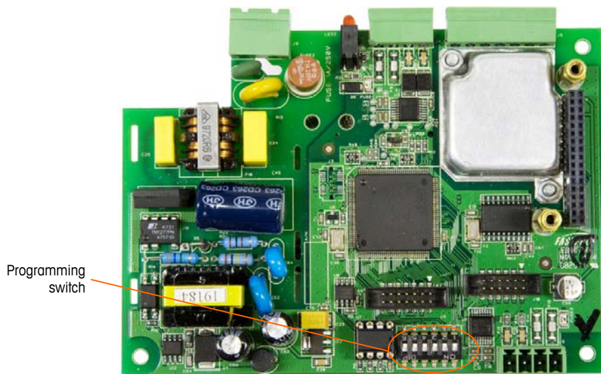
Figure 2-71: Main PCB DIP Switch Array
