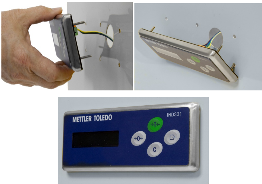
Figure 2-11: Mounting the Operator Interface
