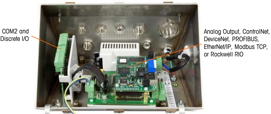
Figure 2-43: Option Locations in the Harsh Enclosure
