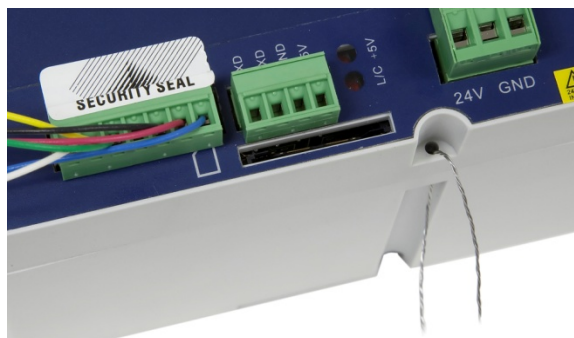
Figure 2-76: DIN and Panel-Mount Sealing – Wire and Paper Seals
