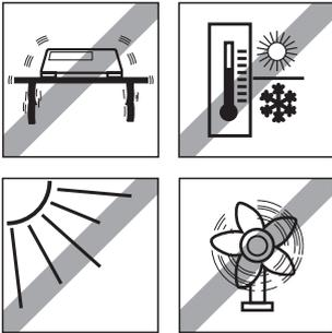
The correct location is crucial to the accuracy of the weighing results.
