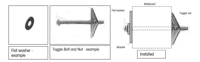
Recommended mounting bolt for wallboard and drywall: Type: Toggle Bolt, 1/4" (6mm), minimum length 2-1/2" to 3" depending on wall thickness, pullout force of 900lb (450kg).
