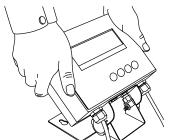
5. Place the XIF indicator on a desk or attach it to a wall with the optional wall-mount bracket. Plug the round connector from the power transformer into the side of the indicator. Plug the power transformer into a 120V AC outlet (indicator can also operate on batteries). To power up the indicator, press the On/Off (PRINT) key and hold it for three seconds.
