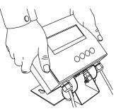
5. Place the XIF indicator on a desk or attach it to a wall with the optional wall-mount bracket. Plug the round connector from the power transformer into the side of the indicator. Plug the power transformer into a 120V AC outlet (indicator can also operate on batteries). To power up the indicator, press the On/Off (PRINT) key and hold it for three seconds.
