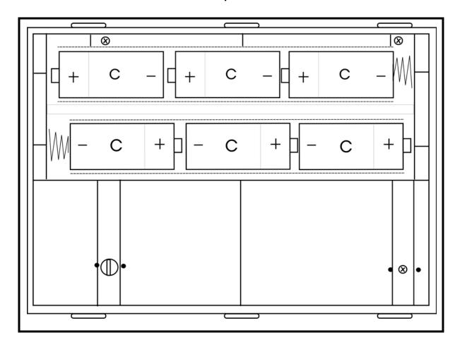
Figure: Shown With Rear Battery Panel Removed
