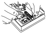
4. Press the front and rear covers together to close the indicator enclosure.
