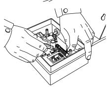
3. Connect the load cell cable to the main PCB according to the cable color code.
