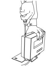
Insert the load cell cable through PG7 connector.
