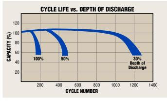
Batteries will last longer if you do not allow them to discharge deeply with each use. MSI recommends recharging within approximately 30% depth of discharge, such as every 12 hours of use for a battery that discharges fully in 40 hours.
