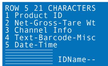
Line preview of a small font entry to line 5. The horizontal bars indicate that a medium font data entry occupies both line 5 and line 6, but in this case, only to the middle of the screen. Therefore a small font entry can be placed on line 5 with a start point at column 11, which allows data with up to 10 characters. This screen also shows, for example, that on line 6, the IDName field is there starting at column 12.
