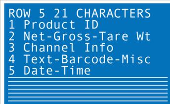
Line preview of a small font entry to line 5. The horizontal bars indicate that a medium font data entry occupies both line 5 and line 6.
