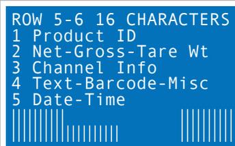
Line preview of a medium font entry. There are small font data items on lines 5 and 6, but a gap exist in the middle. This would allow a 4 character medium font entry with the start column at 9 to fit in. If you want to get rid of all data on lines 5-6, just press **CLEAR**.
