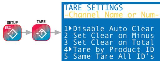
Set Auto Clear Mode with the 1-3 keys. Only 1 item from 1-3 can be enabled at a time. Set the Universal Tare mode with the 4-5 keys.
