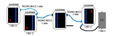
The last load cell will be added to the CellScale scan list as channel four. For information about how to setup the CellScale scan list for this configuration, see the "Software Setup" section.
