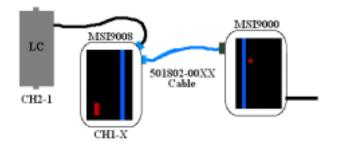
This connection requires the use of the pass thru signal to be used for the ninth load cell. This ninth load cell will be added to the CellScale scan list as channel 2-1. For information about how to setup the CellScale scan list for this configuration, see the "Software Setup section.
