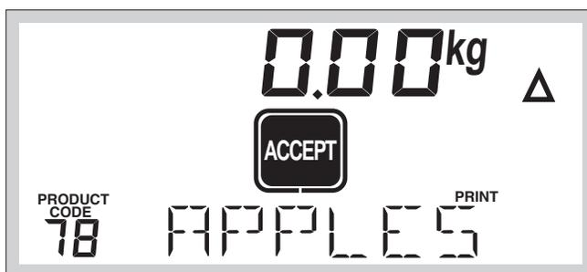
The 6000 LCD showing an Accept target reading in the deviation weight mode.
