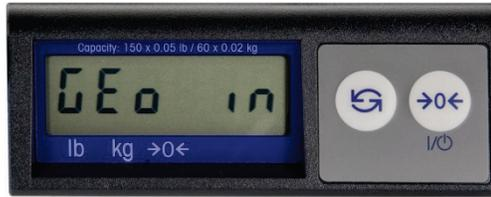
**Figure 2-8: GEOCAL Screen, 7-Segment LCD Display**
