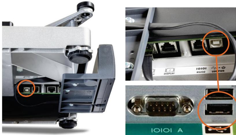
**Figure 2-5: USB Connections, Scale and PC**
