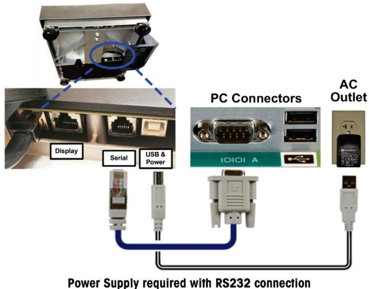
Figure 5-2: Serial Connections
