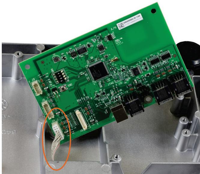
**Figure 5-11: Load Cell Harness Connected to PCB**
