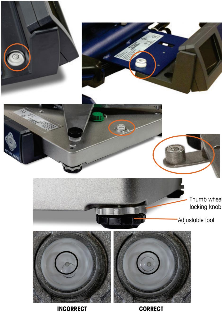
**Figure 2-2: Leveling the Scale**
