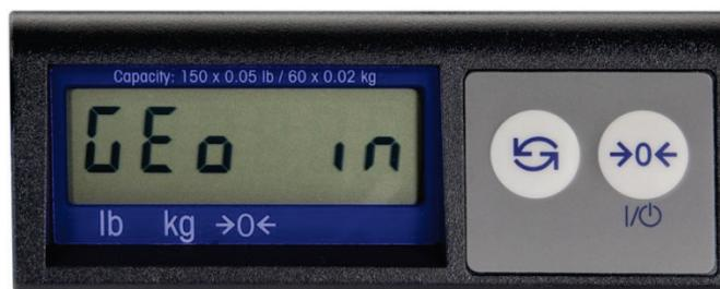
**Figure 4-55: Basic (7-Segment) Display**
