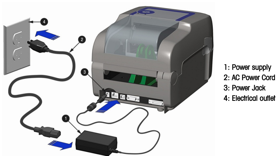
Figure 2-1: Power Connection
