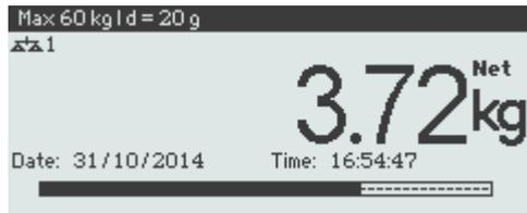
The bargraph indicates roughly which part of the scale capacity is already occupied and what capacity is still available.
