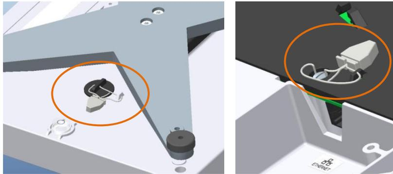
**Figure 4-58: BC-60, -6L, -30 and -3L Sealing**
