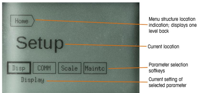
**Figure 3-7: Initial Setup Mode Display**
