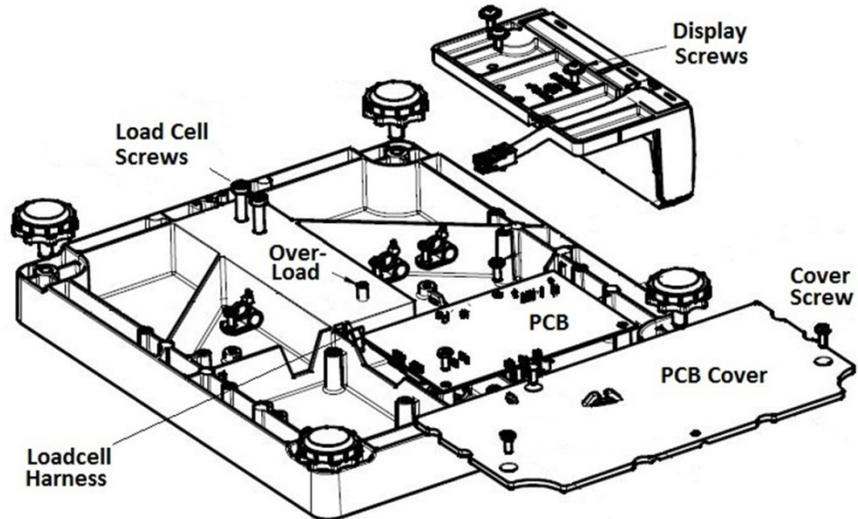
Figure 5-12: Bottom View of Scale
