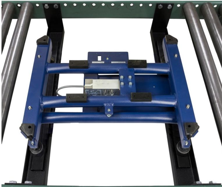
**Figure 2-11: Conveyor Drop-In Kit Installed**
