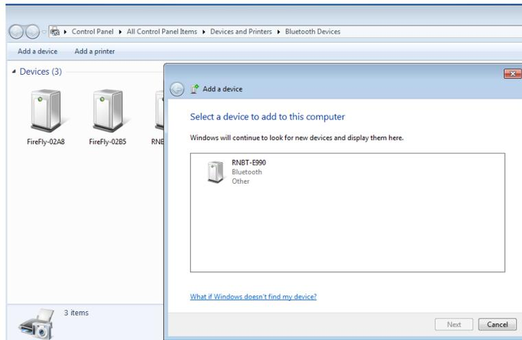
5. Select the device and click **Next**. The PC will try to establish connection with the BT device. If connection is established, the PC will create a pairing code. Click **Next**.
