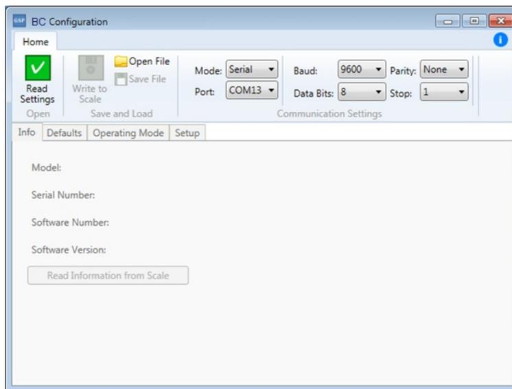
3. The BC Configuration Tool must be able to communicate with the scale. From the **Communication Settings** panel, select the proper parameters.
