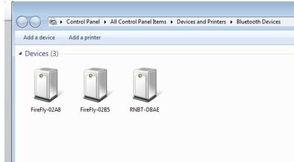
4. Click on the **Add a Device** to add the BC scale BT module. If the BT modules is working correctly, it will appear as a new device.
