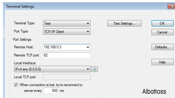
3. Open serial tool like Albatros or Hyperterminal and set the correct Port Type, IP address, and Port setting. Click OK.
