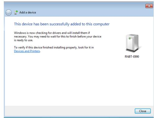
6. Connection is successful and the new device is added to the list of active devices with which the PC can communicate. The PC will install the driver of the BT device and create a virtual COM port.
