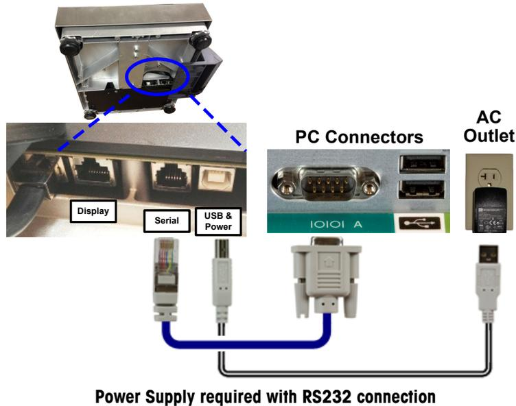
**Figure 5-2: Serial Connections**
