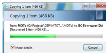
4. Open the file on the PC with the new BC scale software. Copy and paste (drag and drop) the new software file to the BC Firmware folder. The file transfer progress bar will be shown during the download.
