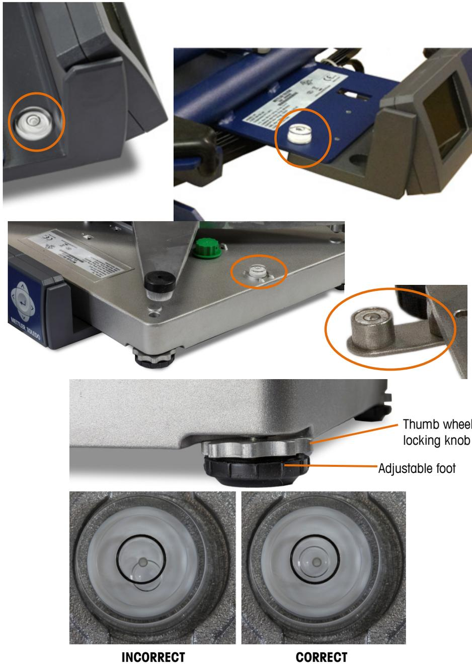
**Figure 2-2: Leveling the Scale**
