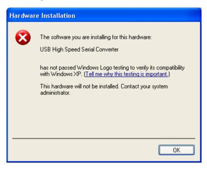
Two options are available to successfully install the device. Either a certified version of the driver can be installed (if available) or the driver signing options can be changed to either warn or ignore to allow the installation to complete.
