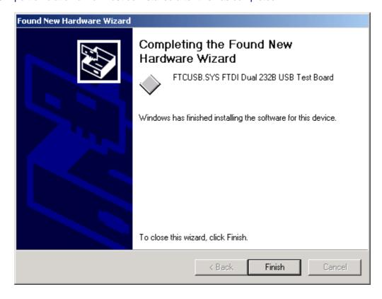
• After clicking "Finish", the Found New Hardware Wizard will continue by installing the COM port emulation driver. Click "Next" to proceed with the serial port installation.
