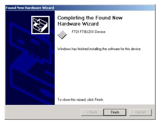
• Open the Device Manager (located in "Control Panel\System" then select the "Hardware" tab and click "Device Manger...") and select "View > Devices by Type". The device appears as a FT8U2XX Device connected to a USB port.
