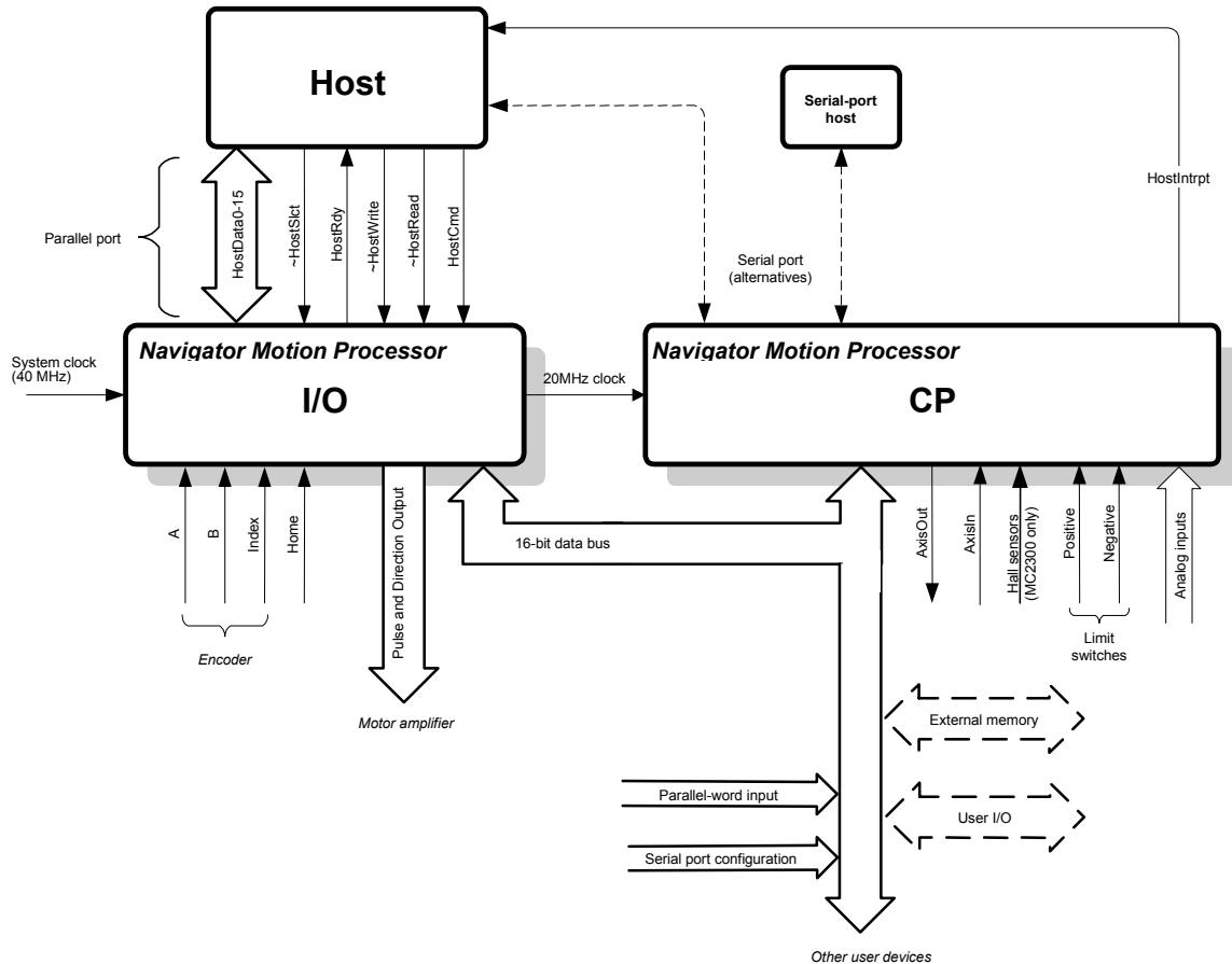
The CP chip contains the profile generator, which calculates velocity, acceleration, and position values for a trajectory. The output of the trajectory generator is used to produce pulse and direction signals that control motor position.
