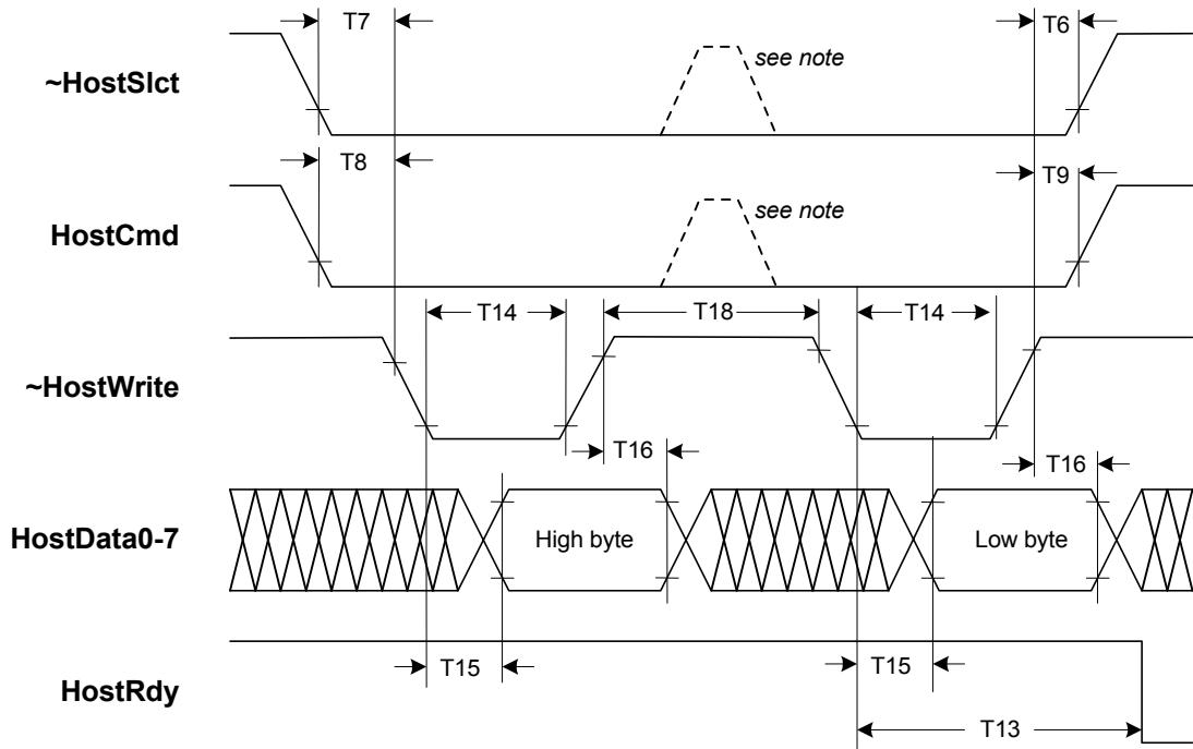
Note: If setup and hold times are met, ~HostSict and HostCmd may be de-asserted at this point.
