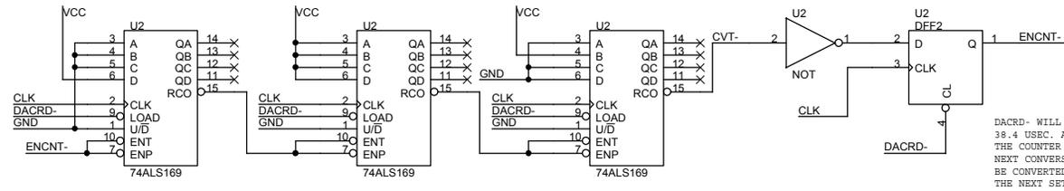
DACRD- WILL LOAD THE COUNTER TO 700. 38.4 USEC. AFTER THE LAST DACRD- THE COUNTER WILL REACH 0 AND START THE NEXT CONVERSION. ALL 4 CHANNELS WILL BE CONVERTED IN 10 USEC. READY FOR THE NEXT SET OF READS AFTER 50 USEC.
