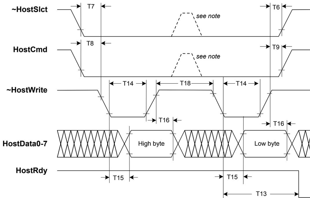
Note: If setup and hold times are met,  $\sim$ HostSlct and HostCmd may be de-asserted at this point.
