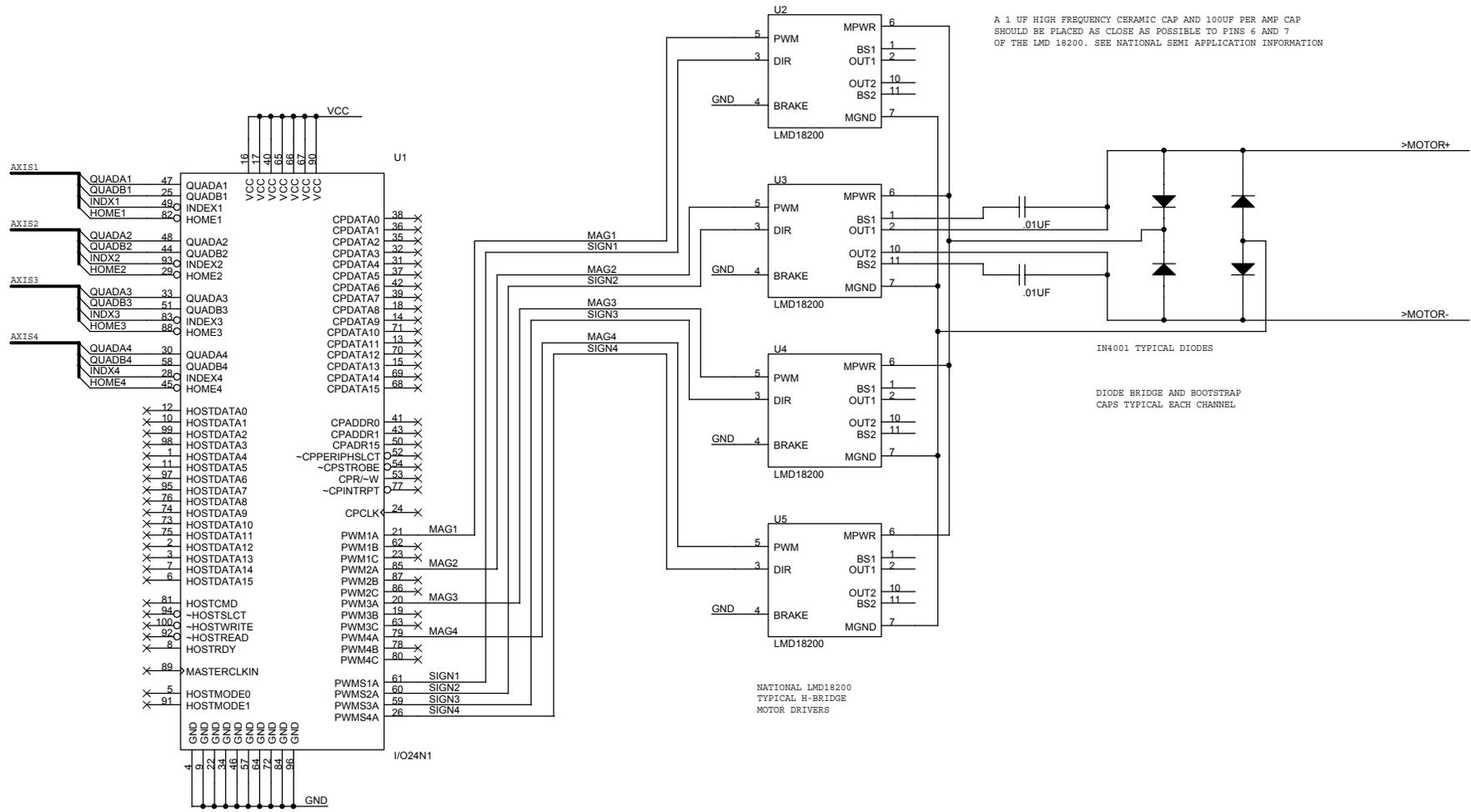
A 1 UF HIGH FREQUENCY CERAMIC CAP AND 100UF PER AMP CAP SHOULD BE PLACED AS CLOSE AS POSSIBLE TO PINS 6 AND 7 OF THE LMD 18200. SEE NATIONAL SEMI APPLICATION INFORMATION
