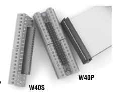
The **W40**<sup>TM</sup> or **W20**<sup>TM</sup> is a low cost Pin-Screw terminal adaptor. W40 converts standard 0.1" lead spacing 20x2 pin headers to 40 screw terminals for easy field wiring. W20 has 20 screw terminals and 20 pins. The **W40P** has a 20x2 pin-header for using a flat ribbon cable. The **W40S** has a 20x2 socket for mounting on top of pin-headers.
