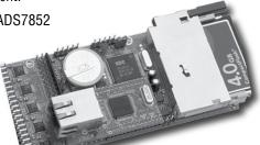
SCA with 48 12-bit High Speed ADCs
