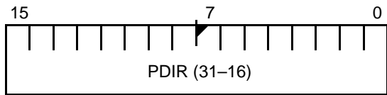
Figure 11-4 PIO Direction 1 Register (PDIR1, offset 78h)
