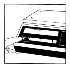
Use the ON/OFF button **(9)** for switching on or off. You can also switch the toploader on with the tare button **(7)**.
