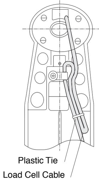
Figure 2-2. Bottom view of MTE Series scale base
