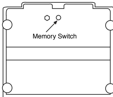
Figure 1-1. Bottom view of NOVA-II scale
