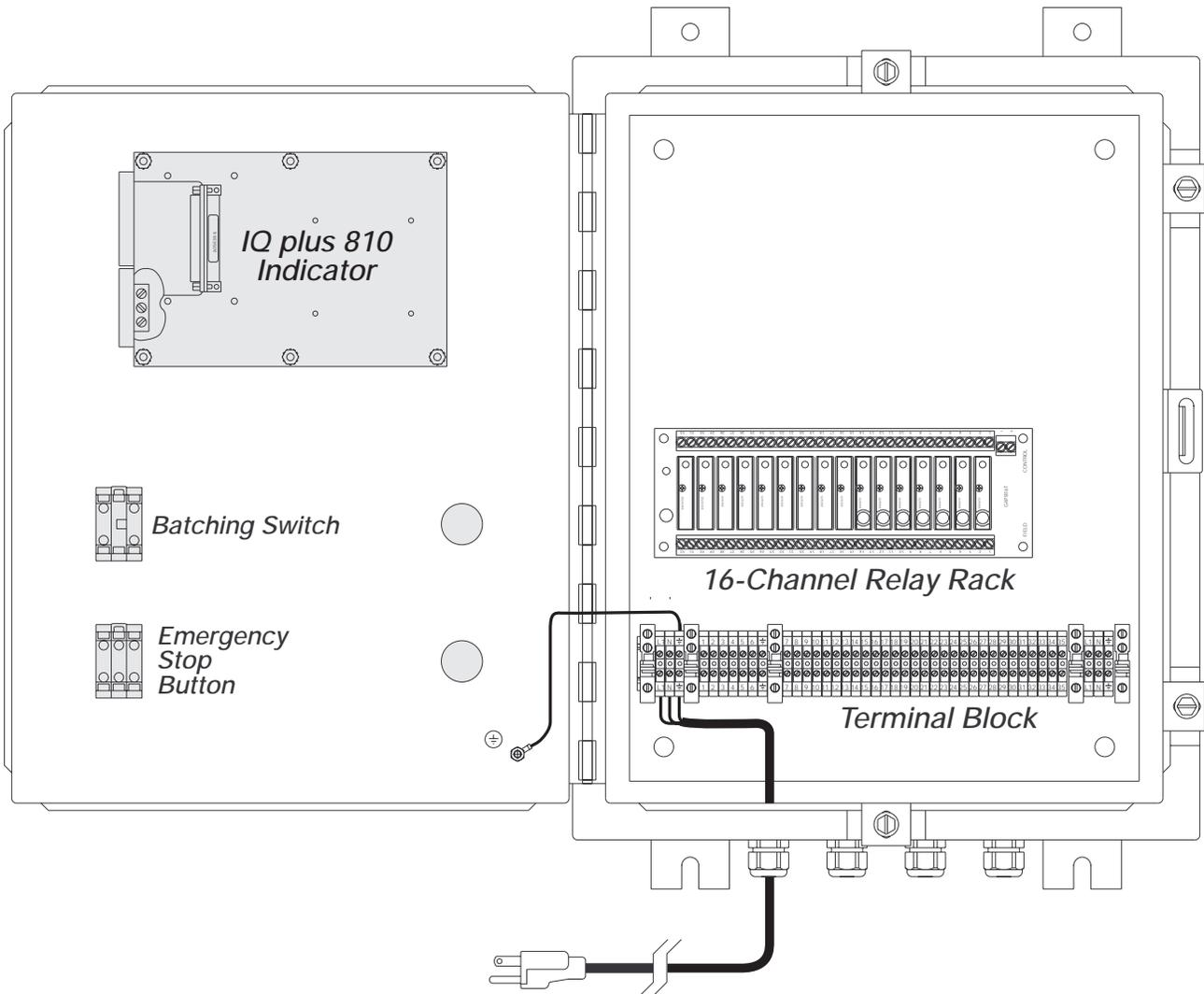
Figure 2-1. BWC-1 Controller Components
