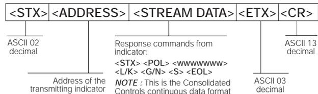
Figure 8-5. RS-485 Continuous Data Format
