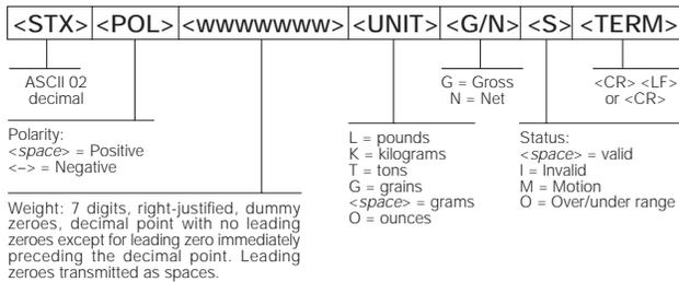
Figure 8-2. Continuous Output Serial Data Format
