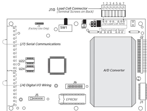
Figure 2-3. CPU Board, Component Side
