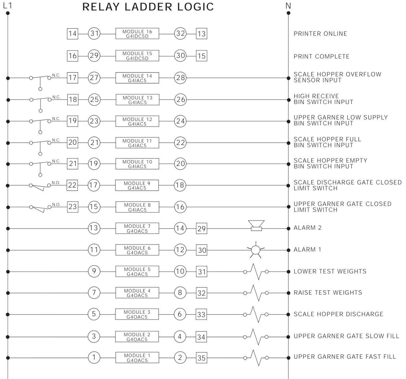
○ Circled numbers refer to connections on the field wiring side of the relay rack
