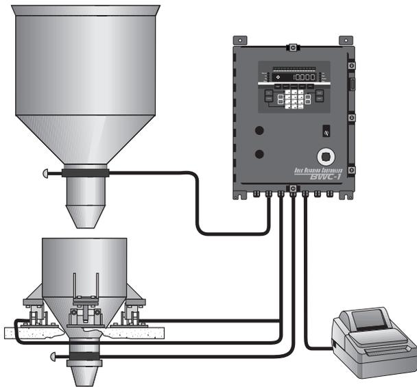
Multidraft weighing provides a method of shipping or receiving a large amount of material by using multiple, smaller drafts of the material. In receive mode, draft weights are accumulated until all material being received has been weighed. In shipping mode, draft weights are accumulated until the target shipping weight has been dispensed.
