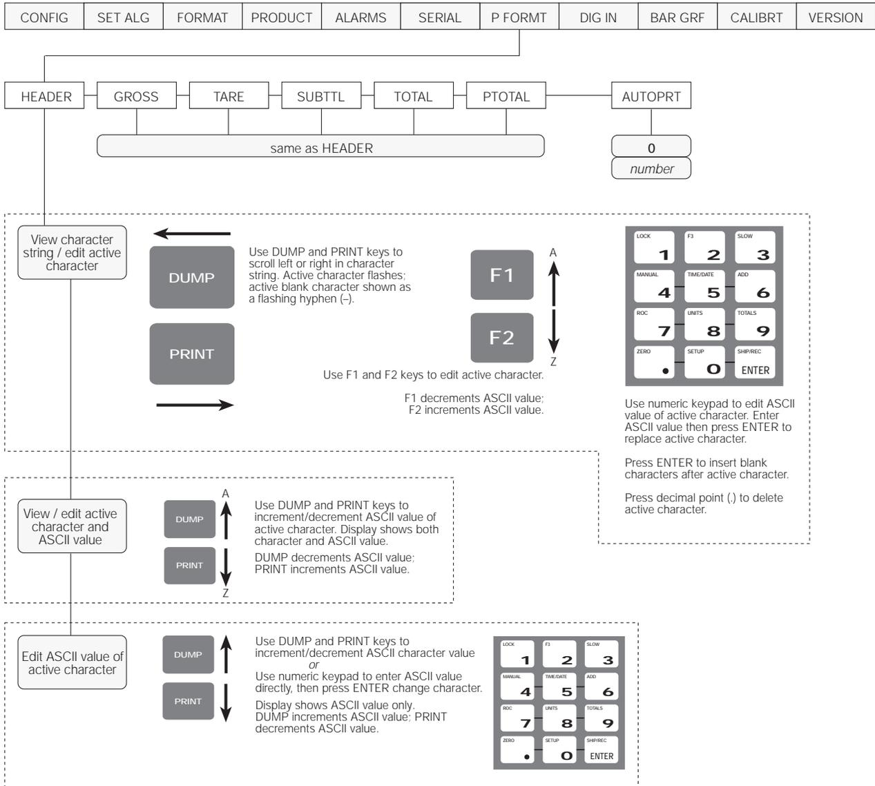
Figure 7-1. P FORMT Menu, Showing Alphanumeric Character Entry Procedure
