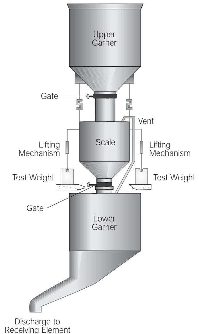
Figure 8-1. Bulk Weighing System with In-Place Test Weights
