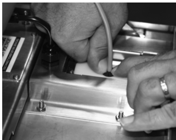
Figure 1-13. Insert Split Grommet Onto the Split Seal Plates
