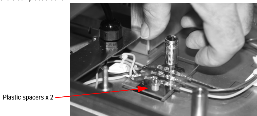
Figure 5-13. Replace Clear Plastic Cover and Gently Tighten
