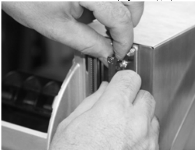
Figure 5-34. Connect the Communications Cable to the Back of the Printer
