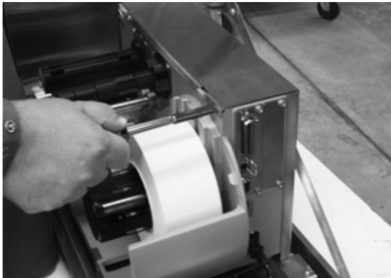
Figure 5-20. Remove Screws from Enclosure
