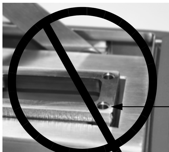
Figure 1-8. Incorrect and Correct Orientation of Main Plate
