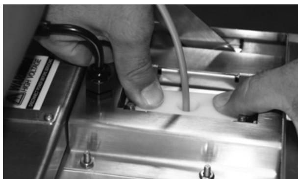
Figure 1-12. Seat the Split Seal Assembly
