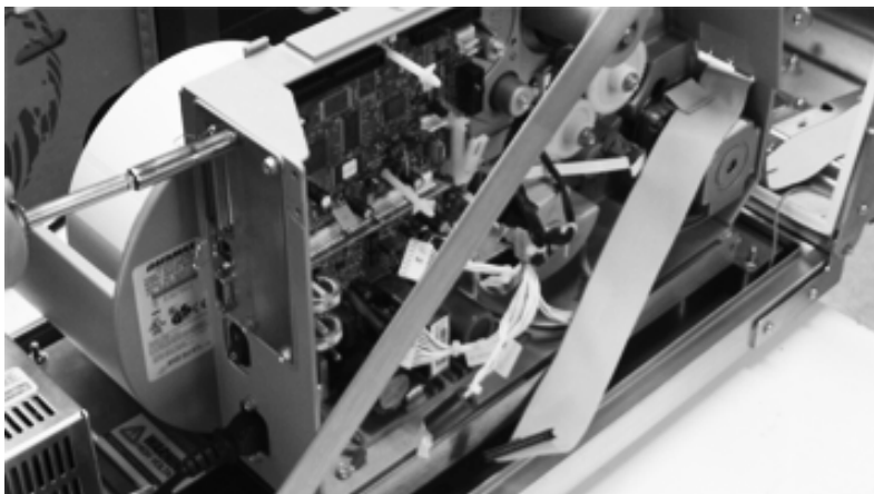
Figure 3-4. Remove Front Panel Screws
