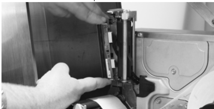
Figure 3-2. Remove Old Printhead Assembly
