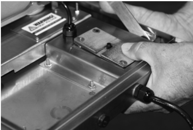
Figure 1-5. Remove the Component Parts of the Split Communications Cable Assembly
