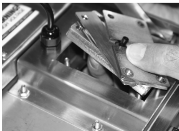
Figure 5-26. Remove the Component Parts of the Split Communications Cable Assembly
