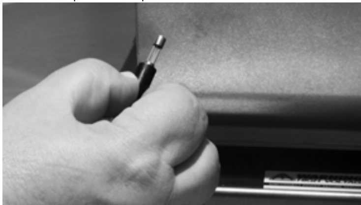
Figure 5-19. Remove Actual Fuse From the Receptacle and Replace with a New Fuse
