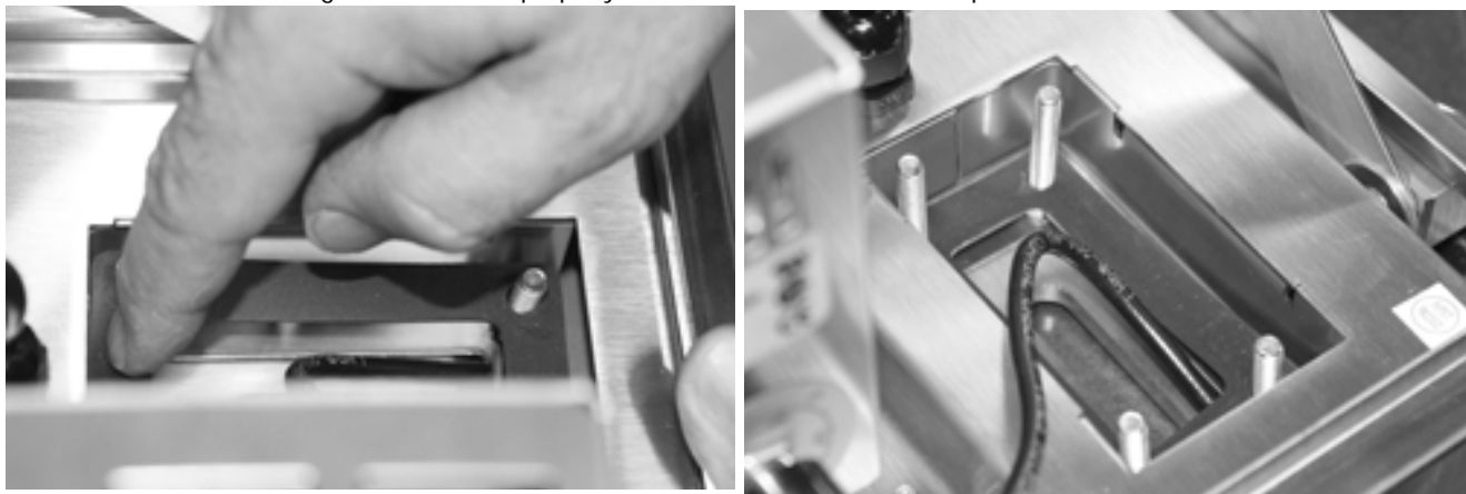
Figure 5-31. Press Down Rubber Gasket Around Bolts
