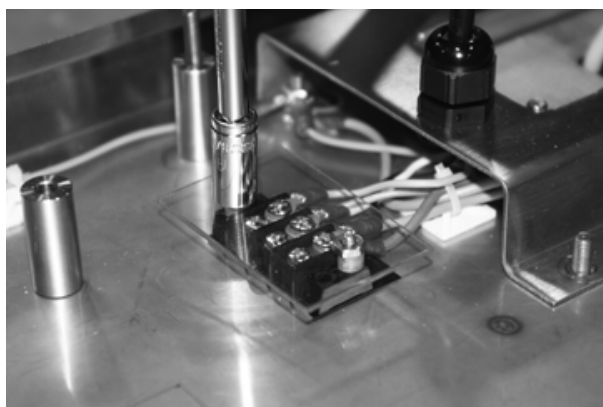
Figure 5-8. Terminal Strip Location, Wiring, and Clear Cover
