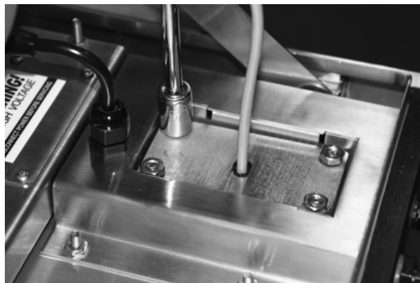
Figure 1-15. Tighten Up The Entire Assembly
