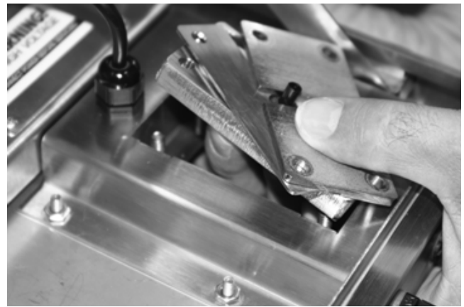
Figure 1-5. Remove the Component Parts of the Split Communications Cable Assembly
