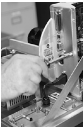
Figure 5-21. Remove Screws from Cover Plate
