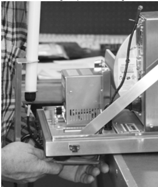
Figure 5-30. Installing Antenna Kit Bolts and Cable Through Printer Base
