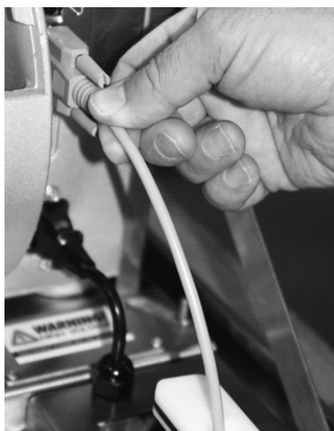
Figure 1-11. Connect Communications Cable to Back of Printer
