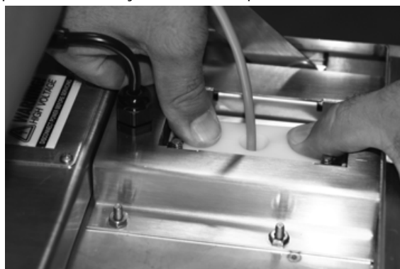
Figure 5-35. Seat the Split Seal Assembly
