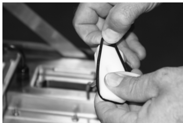
Figure 1-10. Assemble Split Seal Plates Together
