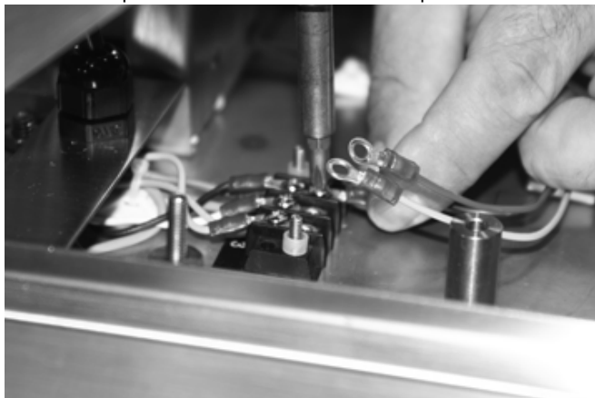
Figure 5-11. Color Match Wire Harness and Terminal Strip Wires
