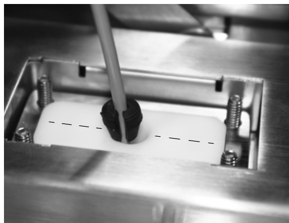
Figure 1-13. Insert Split Grommet Onto the Split Seal Plates
