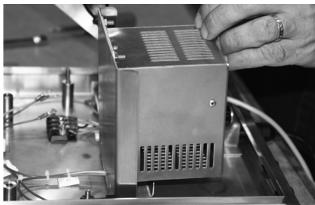
Figure 5-10. Secure Heater to Enclosure Bottom
