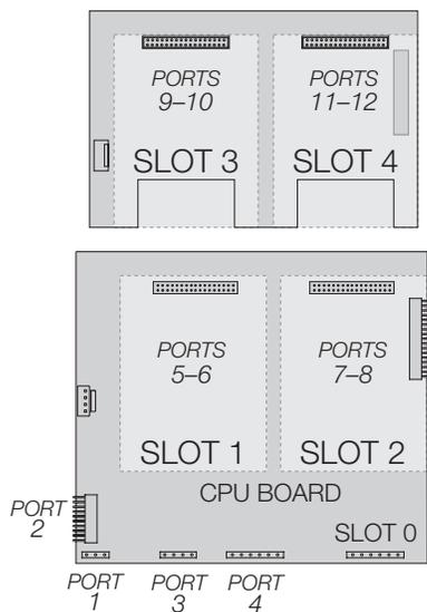
Figure 2-11. Serial Port Assignments, Two-Card Expansion Board
