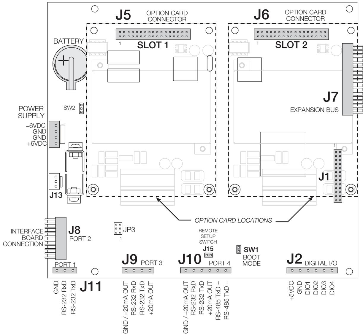
Figure 2-5. 920i CPU Board, Showing Option Card Locations
