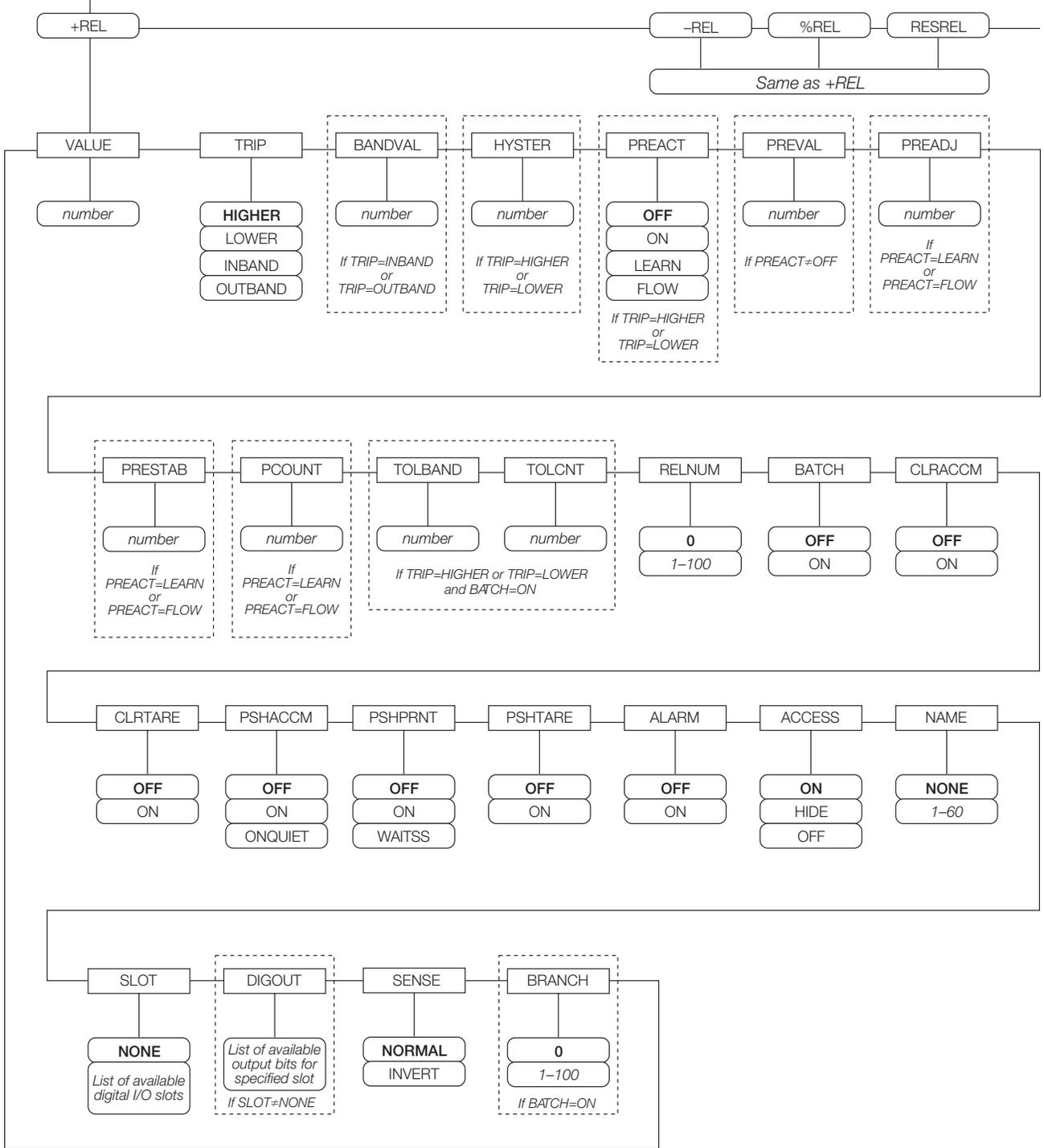
Figure 8-3. +REL, -REL, %RELS and RESREL Setpoint Parameters
