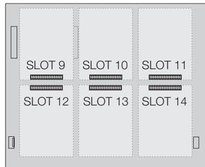
Figure 2-10. CPU Board with Two Six-Card Expansion Boards
