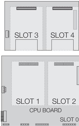
Figure 2-8. CPU Board with Two-Card Expansion Board
