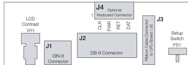
Figure 2-4. Interface Board, Top View
