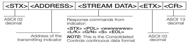
Figure 10-5. RS-485 Continuous Data Format
