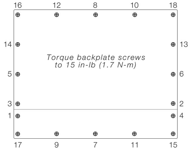
Figure 2-12. 920i Enclosure Backplate
