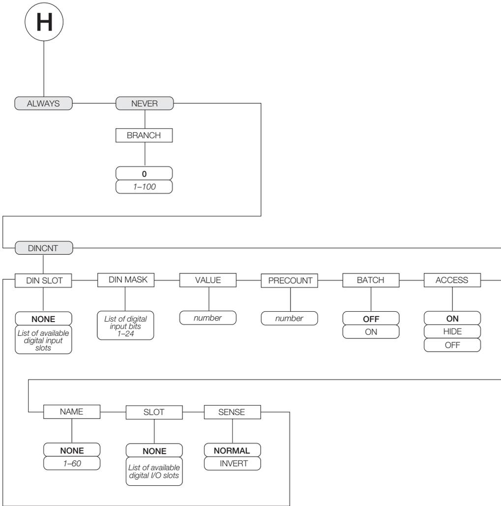
Figure 8-9. ALWAYS, NEVER, and DINCNT Setpoint Parameters
