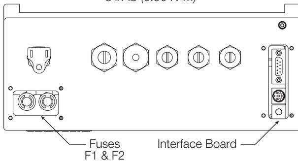
Figure 2-13. Interface Board and Fuse Locations, Universal Model
