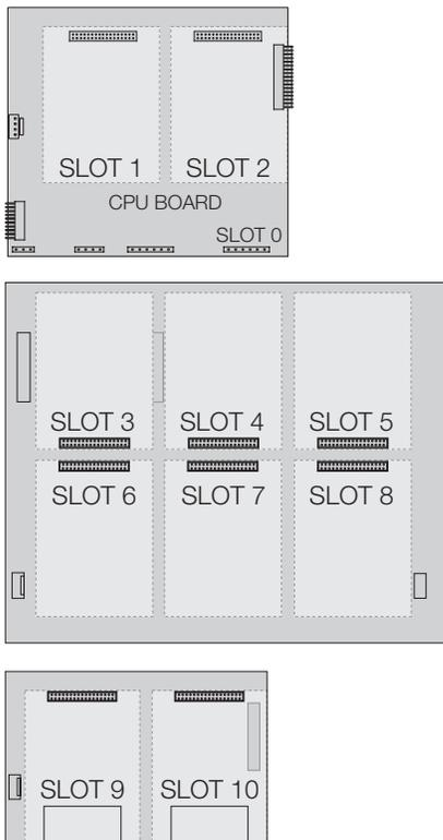
Figure 2-9. CPU Board with Two- and Six-Card Expansion Boards
