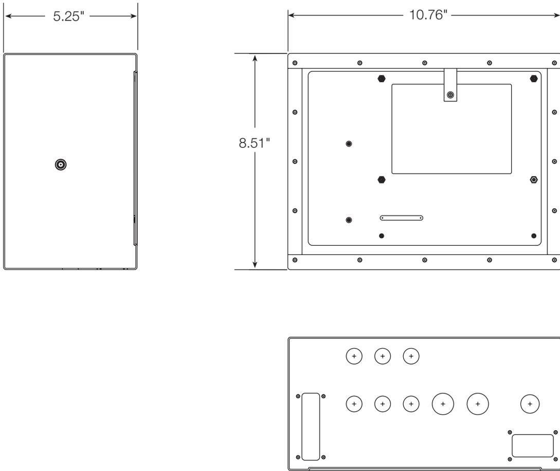
Figure 10-7. Deep Enclosure Model Dimensions
