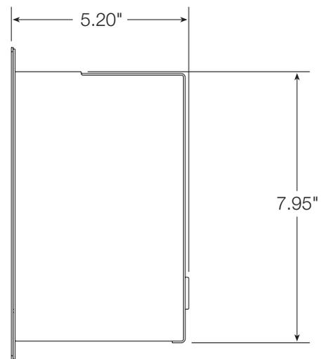
Figure 10-8. Panel Mount Model Dimensions
