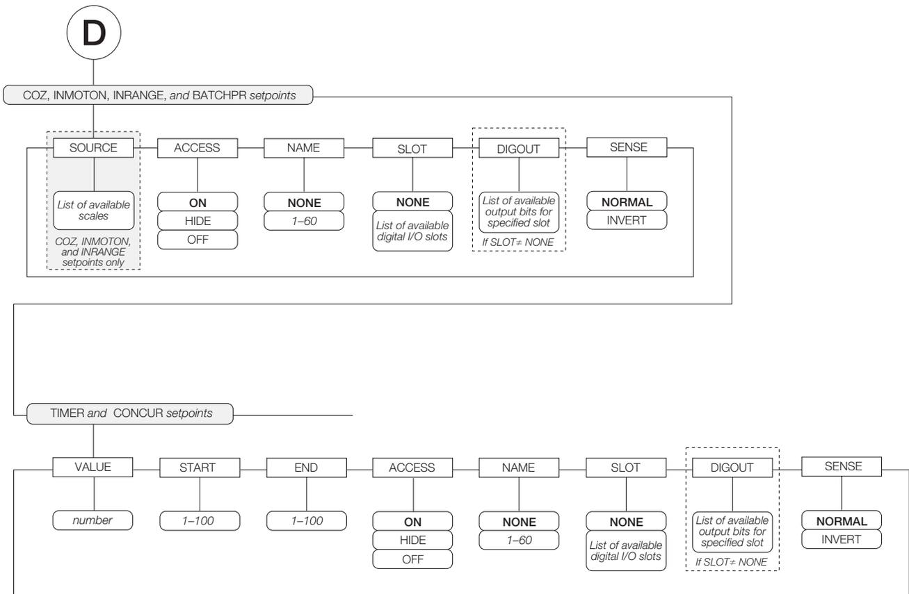
Figure 8-5. COZ, INMOTON, INRANGE, and BATCHPR Setpoint Parameters
