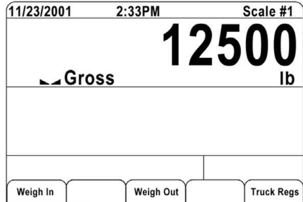
Figure 7-1. 920i Display, showing Truck Mode Softkeys
