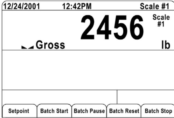
Figure 8-10. Batching Softkeys
