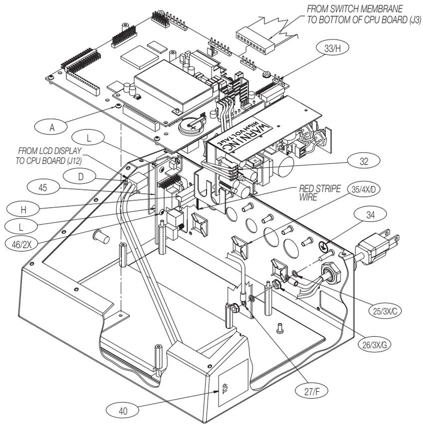
Figure 2-15. 920i Universal Model CPU Board and Power Supply Components
