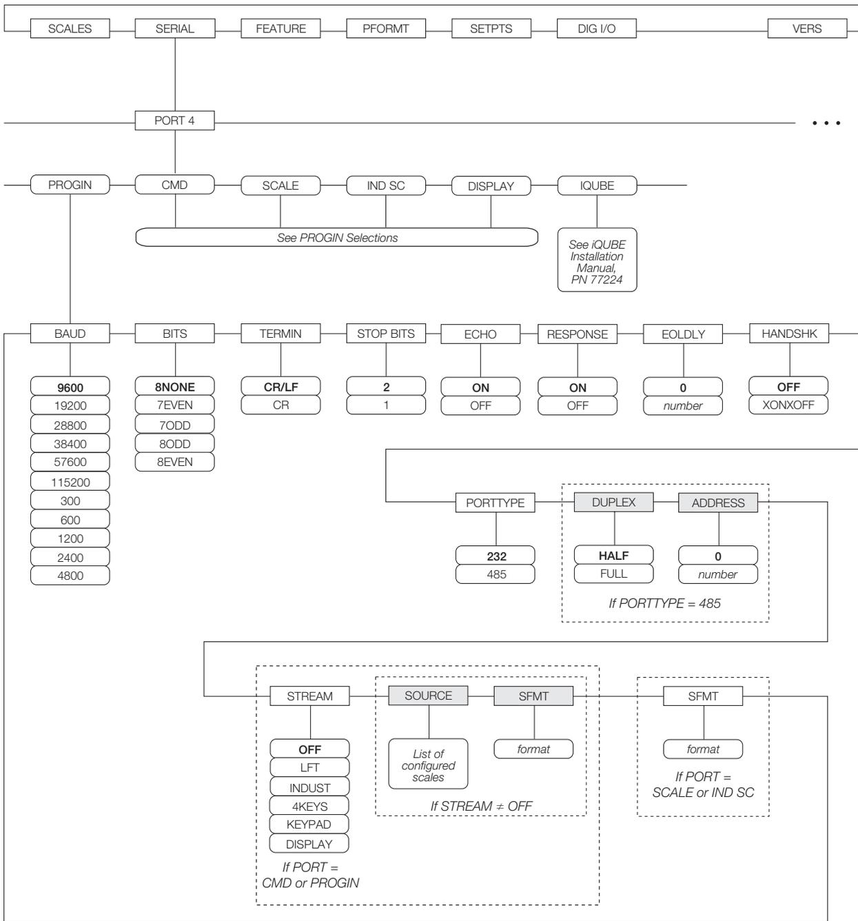
Figure 3-10. SERIAL Menu, Port 4 and Expansion Ports
