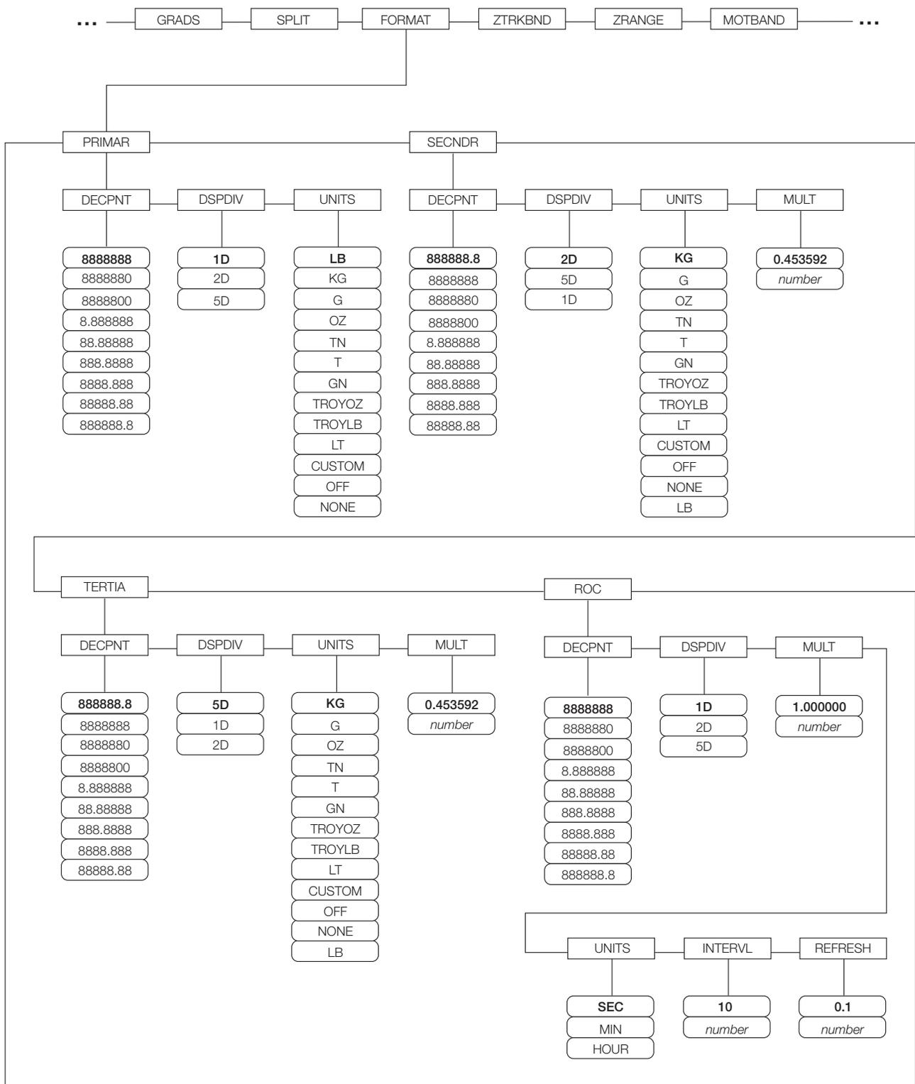
Figure 3-5. SCALES Menu, FORMAT Submenu, SPLIT = OFF
