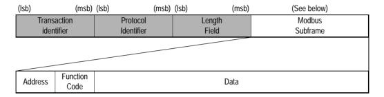
Note that the Modbus/TCP message frame does not include a CRC field as Modbus does, since the TCP/IP frame format already features sophisticated error checking.
