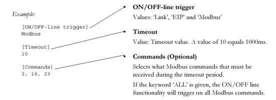
The headings '[Timeout]' and '[Commands]' shall only given if the ON/OFF-line Trigger value is set to 'Modbus'.
